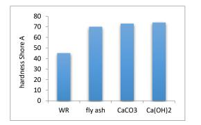
Fig (4) Hardness for different filler types and for WR filler.
