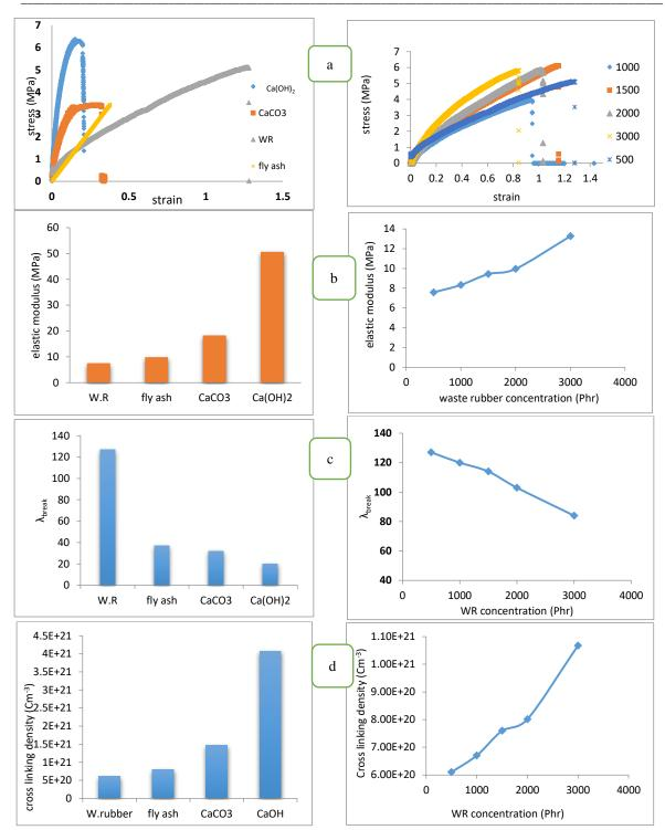
**Fig (3) mechanical measurements results (a) Stress** Strain curve for the different filler types and the different WR filler. (b) Elastic Modulus for the different filler types and for the WR filler. (c) Elongation at break for the different filler types and for WR filler. (d) Cross linking density for different filler types and for WR filler
