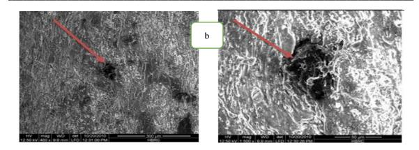
Fig (1) a) Specific gravity for different filler types and different W. rubber concentrations. b) SEM image indicate the air pores.
