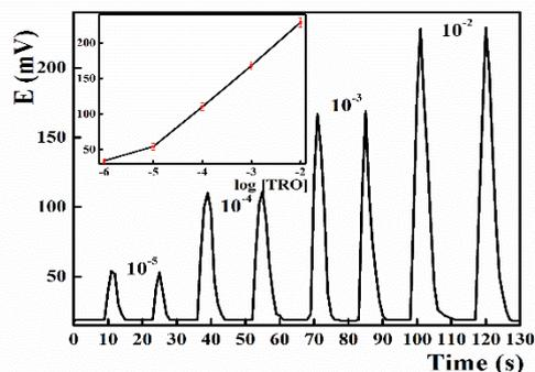
Fig. 7: FIA potentiometric determination of TRO using  $\alpha$ -CD/MWCNTs screen printed sensors.
