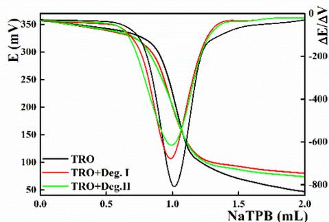
Fig. 8: Potentiometric titration of 3.92 mg TRO in presence of its degradation products against  $10^{-2}$  mol L<sup>-1</sup> NaTPB.
