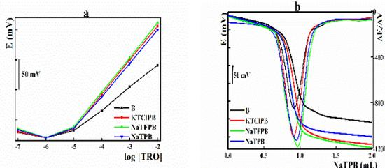
**Fig.2.** Effect of the ionic sites on: a) TRO sensor performance; b) potentiometric titration of 1 ml of 10<sup>-2</sup> mol L<sup>-1</sup> TRO with 10<sup>-2</sup> mol L<sup>-1</sup> NaTPB solution.
