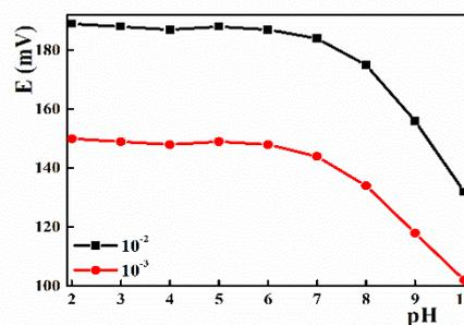
**Fig. 5 : Effect of the pH on TRO sensor potential reading**
