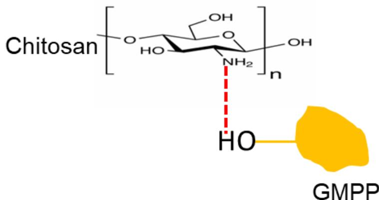
Fig. 5. Schematic diagram representing the interaction between GMPP and Chitosan chains
