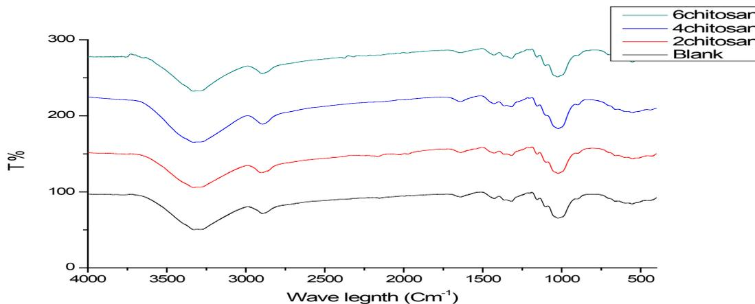
Fig(3a). FT-IR of the treated Shibeka fabrics treated with different chitosan concentration.
