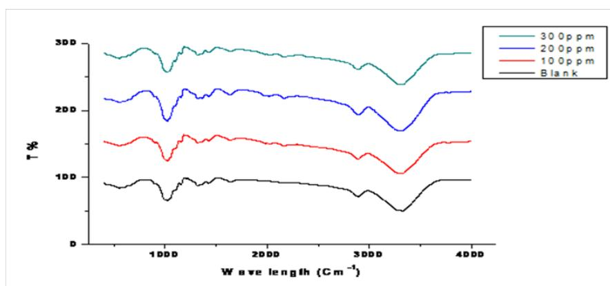
Fig (3b). FT-IR of the treated Shibeka fabrics treated with different silver concentration .
