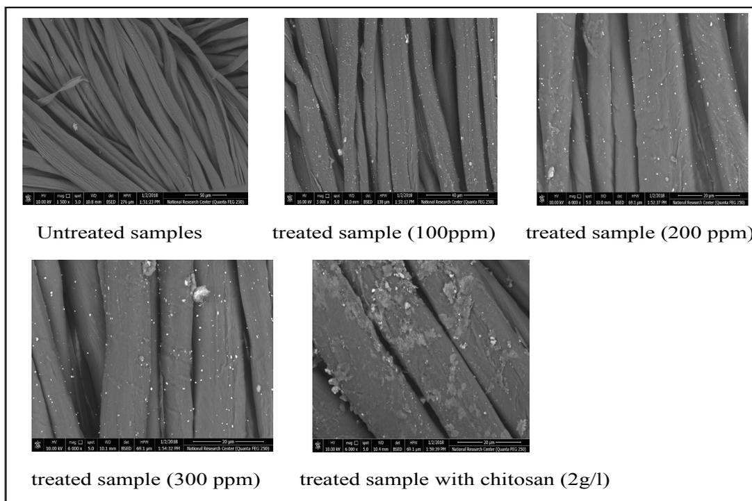
Fig.4. SEM images of the treated Shibeka fabrics with different AgNPs concentration and chitosan (2g/l).
