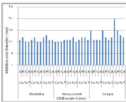
Fig. 1. Antibacterial properties of fabrics treated with chitosan.
