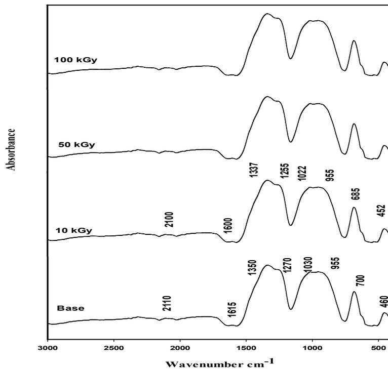
Fig. 5. Infrared absorption spectra of the base glass before and after gamma irradiation.
