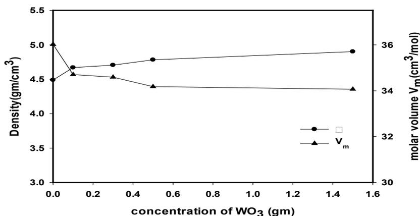
Fig. 2. Density and molar volume of  $PbO$ – $B_2O_3$ – $WO_3$  glasses.
