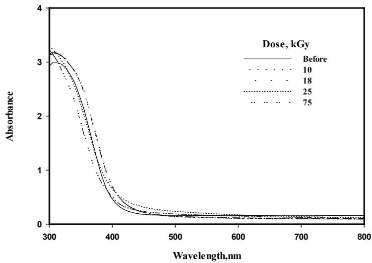
Fig. 9. UV-visible absorption spectra of undoped lead borate glass before and after successive gamma irradiation.
