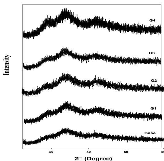
Fig. 1. XRD pattern for lead borate glass doped with different concentrations of  $WO_3$
