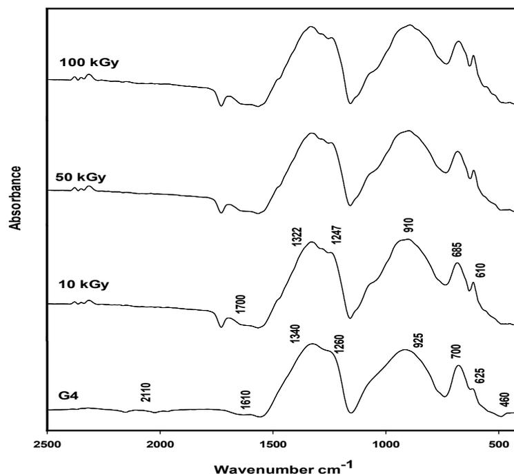
**Fig. 7.** Infrared absorption spectra of the lead borate glass doped with  $\text{WO}_3$  (G4) before and after gamma irradiation.
