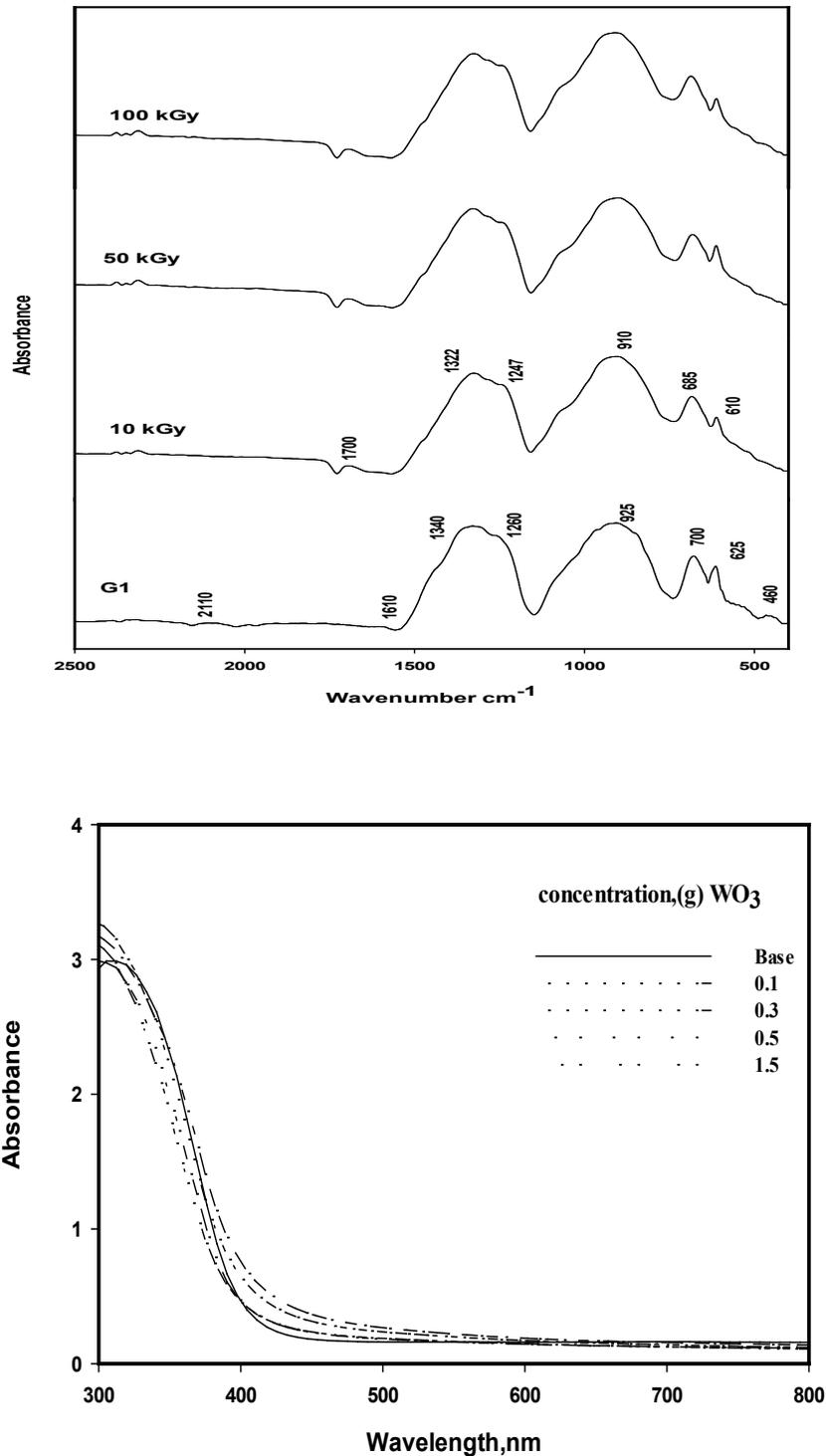
Fig. 8. UV-visible absorption spectra of undoped and doped lead borate glass with different concentrations of WO<sub>3</sub>.
