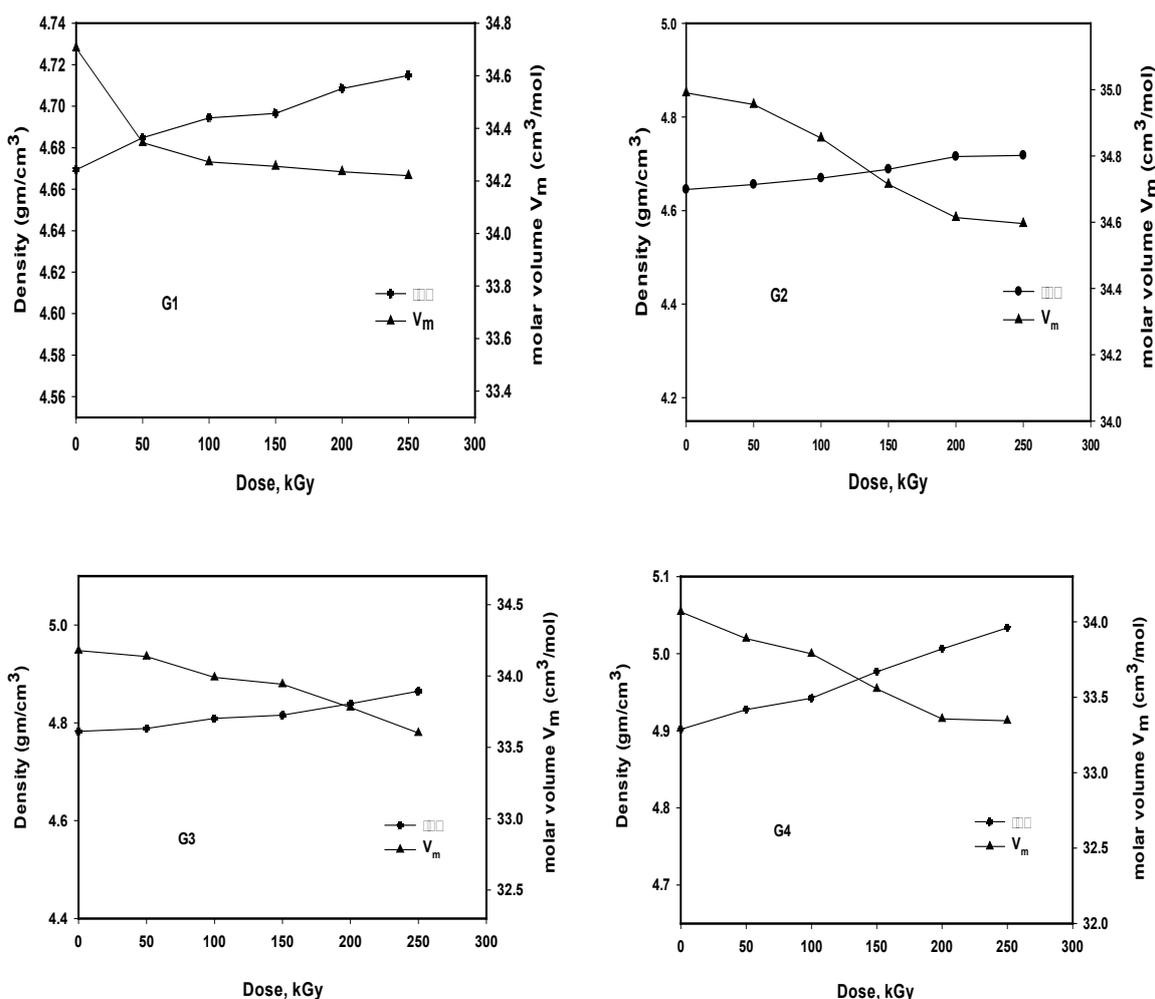
Fig. 3. Density and molar volume of  $PbO-B_2O_3-WO_3$  glasses (G1-G4) after gamma irradiation.
