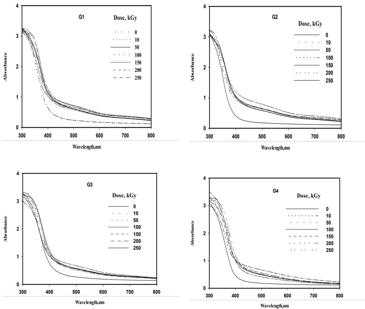
Fig.10. Optical absorption spectra of WO<sub>3</sub>-doped lead borate glasses with increasing WO<sub>3</sub> contents before and after gamma irradiation.
