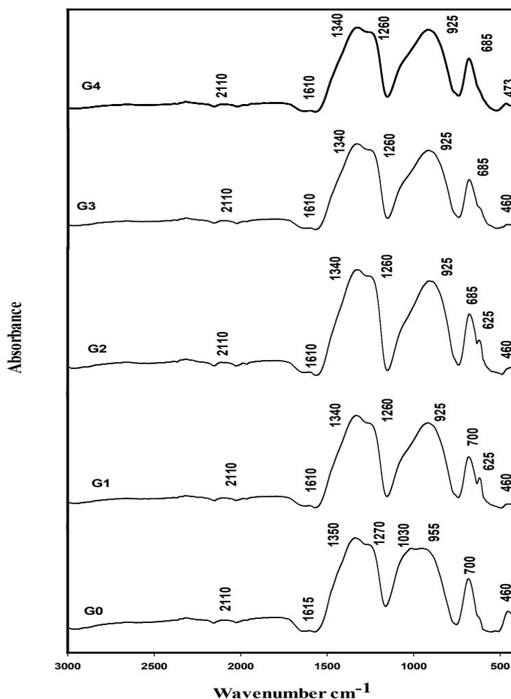
Fig. 4. Infrared absorption spectra of lead borate glass doped with different concentrations of  $\text{WO}_3$ .
