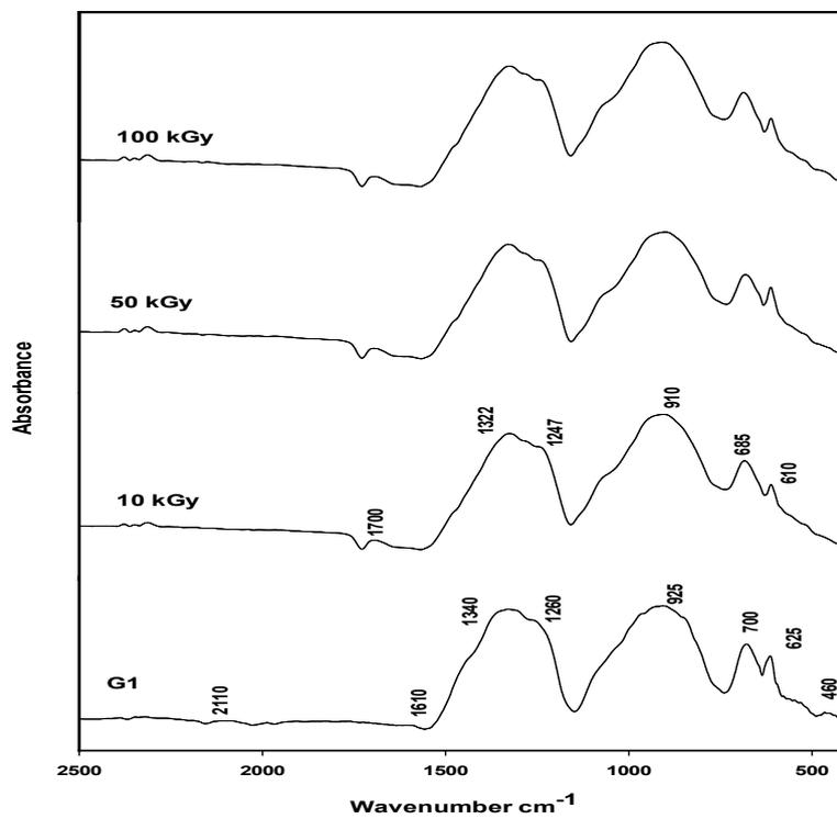
Fig. 6. Infrared absorption spectra of the lead borate glass doped with  $\text{WO}_3$  (G1) before and after gamma irradiation
