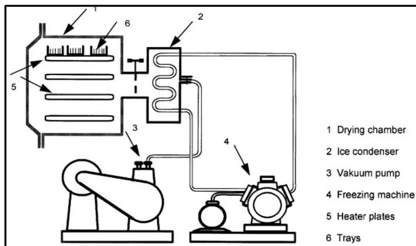
Fig. 24. Freeze-drying [75].
