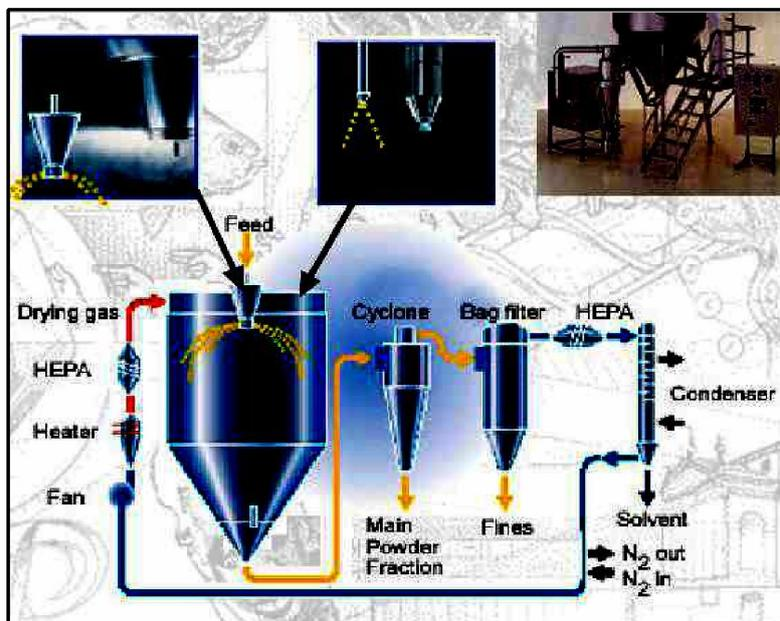
Fig. 17. Schematic illustrating the process of encapsulation by spray-drying [58].
