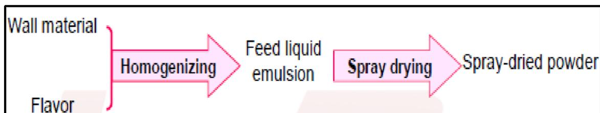
Fig. 12. Preparation of spray-dried powder [68] .
