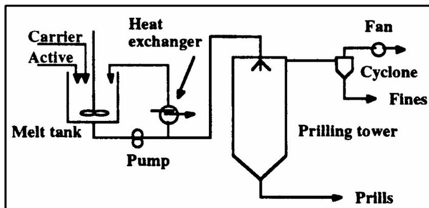
Fig. 23. Spray chilling (Prilling) [53].
