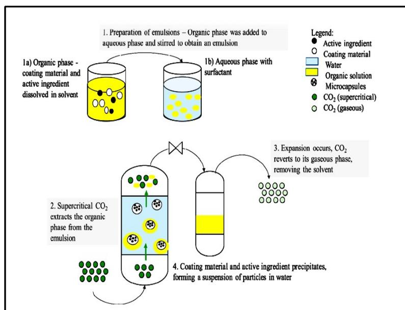
Fig. 11. Schematic representation of supercritical fluid extraction of emulsions (SFEE) [61].
