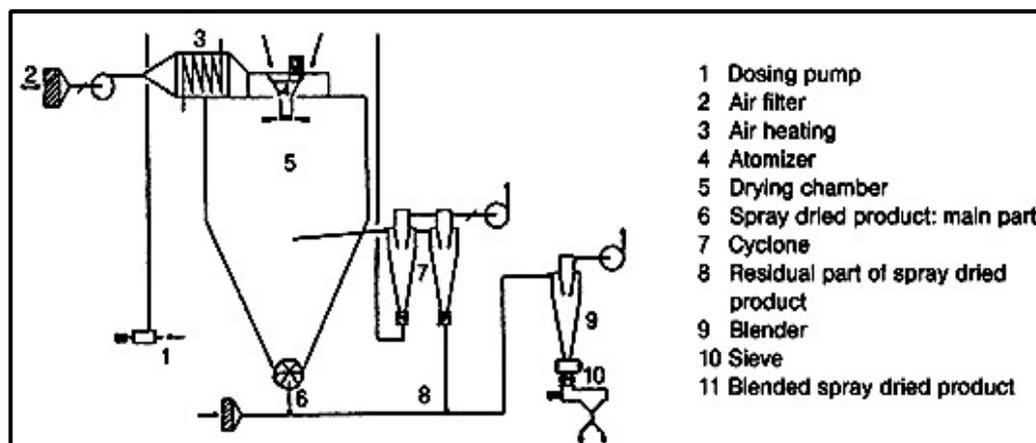
Fig. 13. Principle of a spray drying plant [58].
