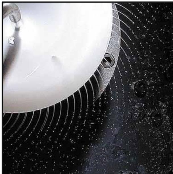
Fig. 28. Encapsulation by spinning disc [12,25].
