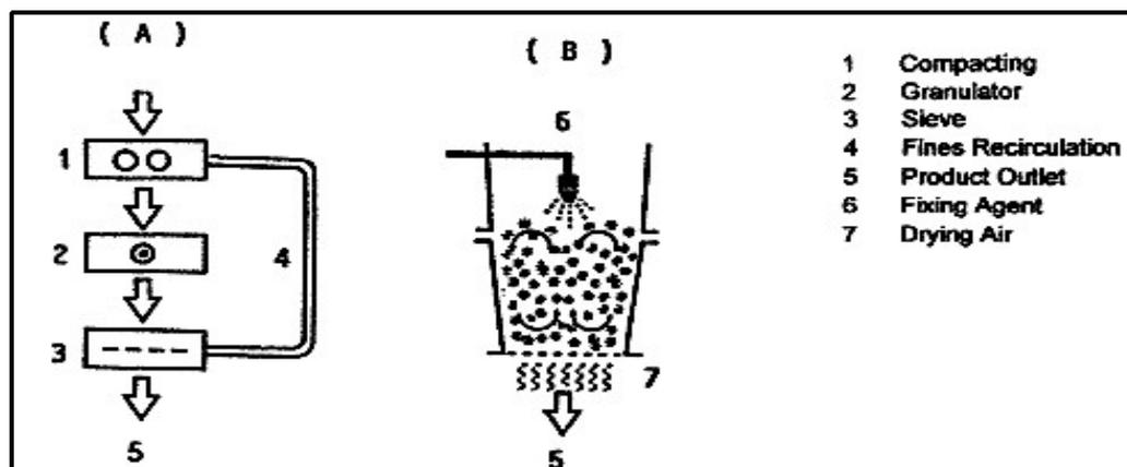
Fig. 19. Principle of plant compacted products (A) and agglomerated products (B) [58].
