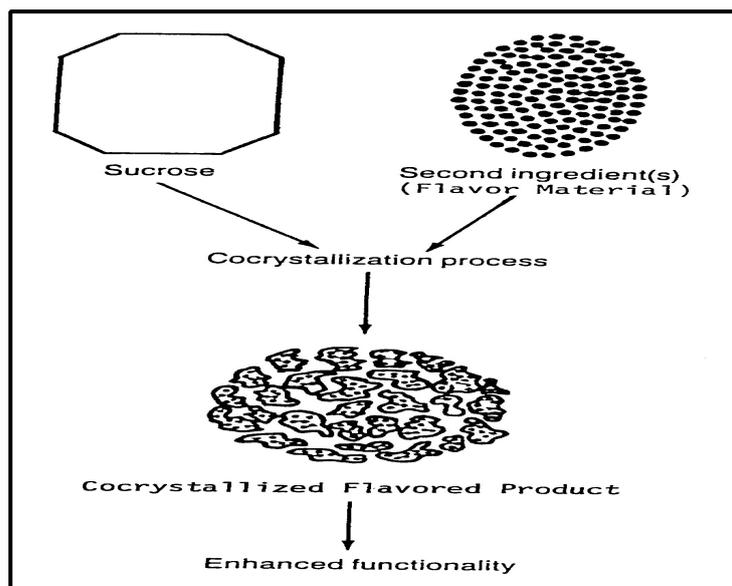
Fig. 29. Flow diagram of encapsulation cocrystallization process [83].
