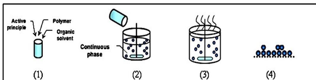
Fig. 9. Basic steps of microencapsulation by solvent evaporation [60].
