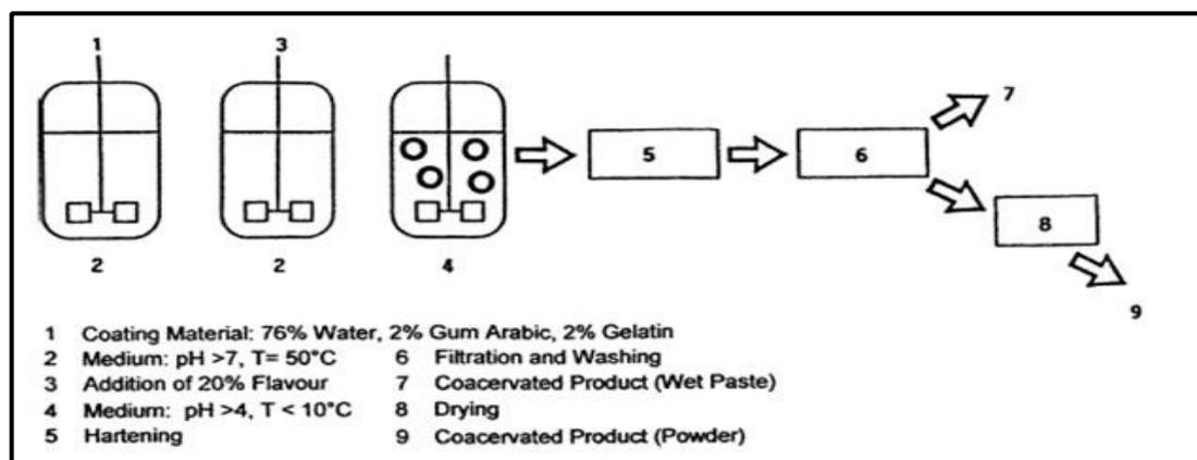
Fig. 7. Principle of a coacervation plant [58].
