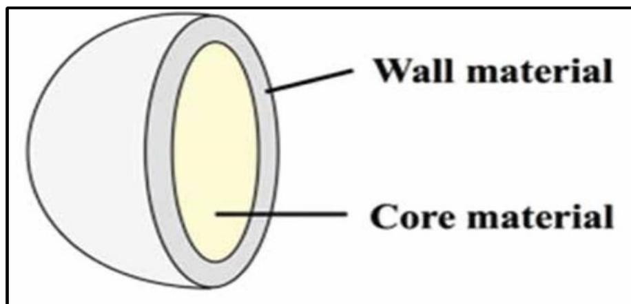
Fig. 1. Schematic presentation of the capsule structure [8].
