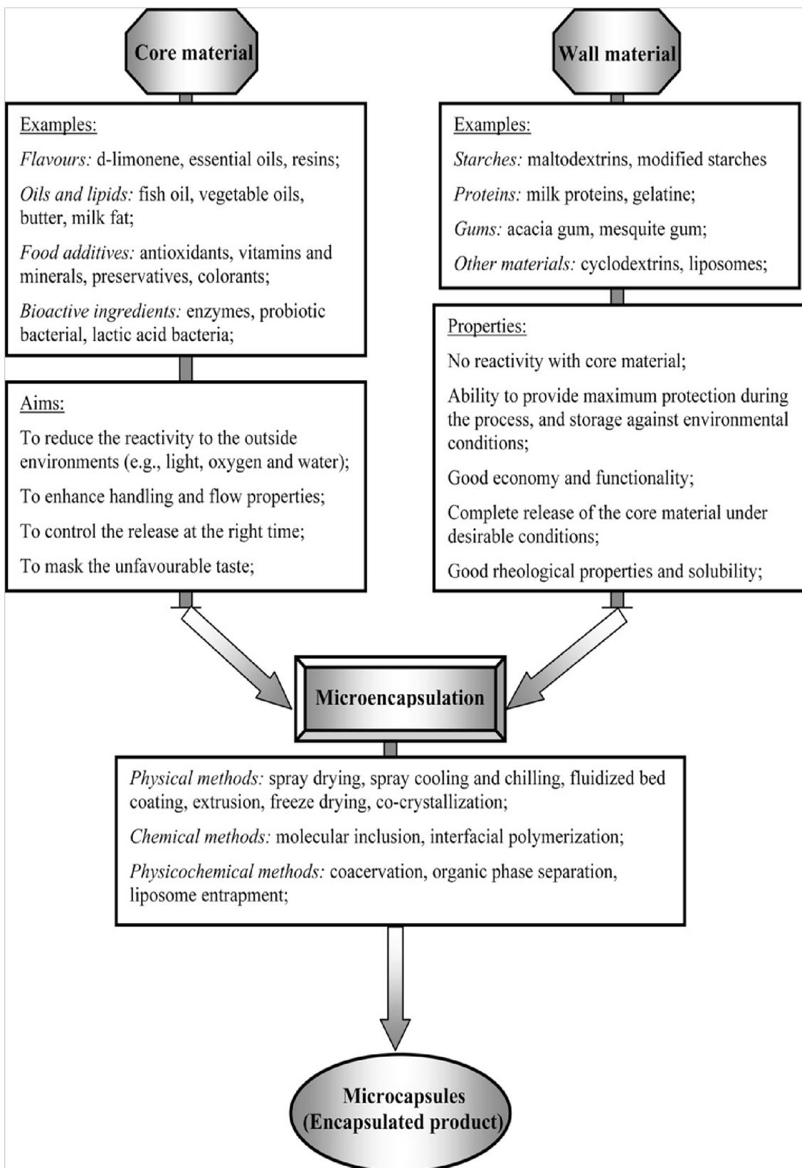
Fig. 3. Schematic description of the microencapsulation of food ingredients along with some examples of core and wall materials, wall material properties, aims, and different techniques of the microencapsulation [38].
