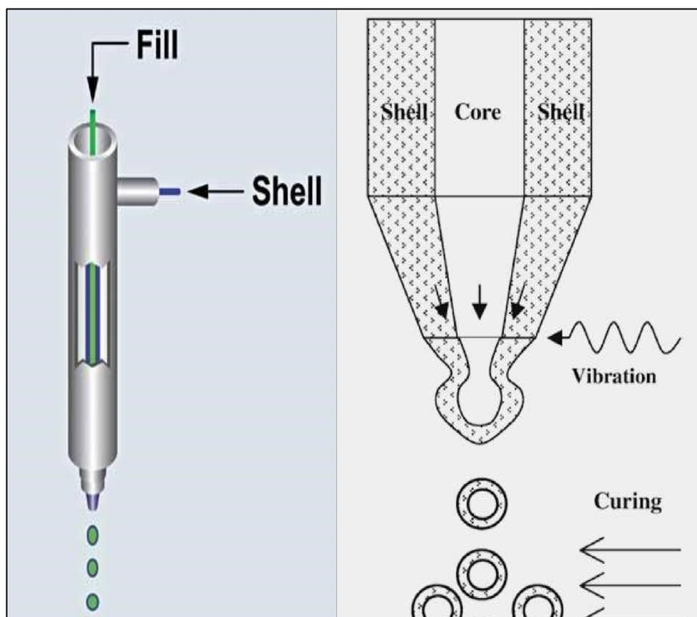
Fig. 27. The Co-extrusion process [81].
