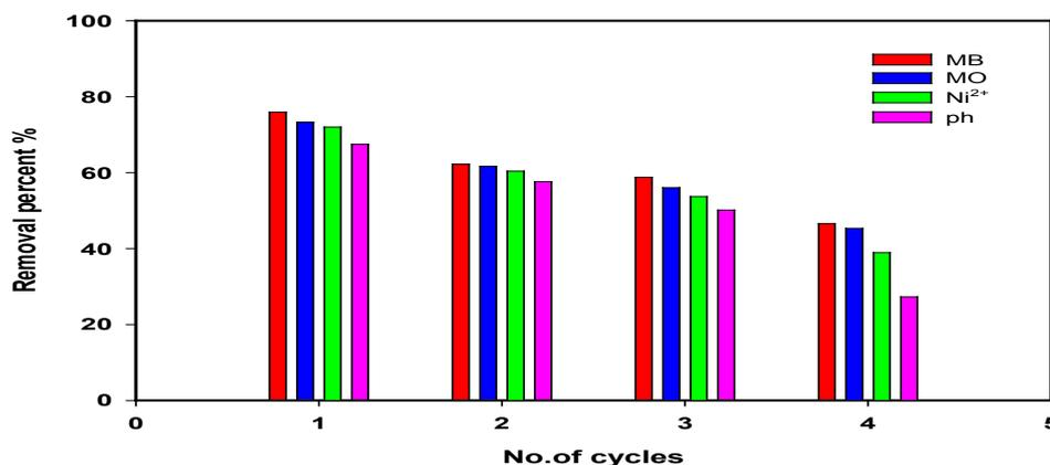
Fig. 12. Effect of adsorption–desorption cycles on adsorption capacities of ACPP in the removal of all pollutants from wastewater
