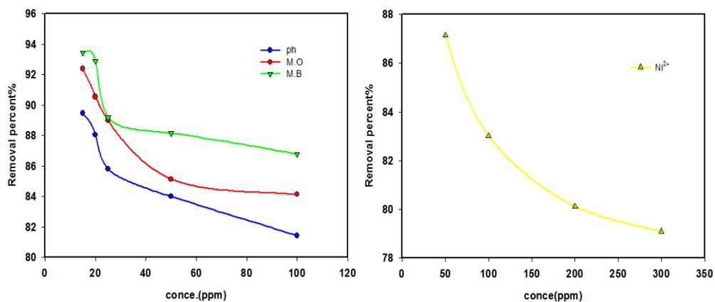
Fig. 7. Effect of initial concentration on removal percent of pollutants at contact time; 150 mint., medium pH; 4 for (Ni<sup>2+</sup>, MO), 9 for (MB), 7 for (Ph) Temperature; 80°C, and adsorbent dose; 1g.
