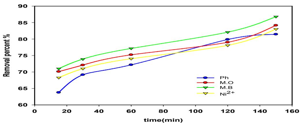
Fig. 4. Effect of time on removal percent of pollutants at initial concentration; 100 ppm, medium pH;4 for (Ni<sup>2+</sup>,MO), 9 for (MB), 7 for (Ph) Temperature; 80°C and dose;1g
