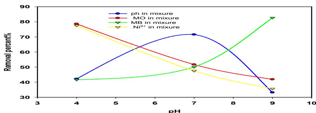
Fig. 11. Effect of medium pH on removal percent of pollutants in mixture at initial concentration; 100 ppm, dose; 1g, Temperature; 80 °C, and contact time;150 min.
