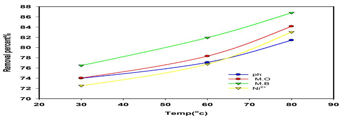
Fig. 9. Effect of temperature on the removal percent of pollutants at initial concentration; 100 ppm, at contact time; 150 min., medium pH; 4 for ( $Ni^{2+}$ , MO), 9 for (MB), 7 for (Ph) and adsorbent dose; 1 g.
