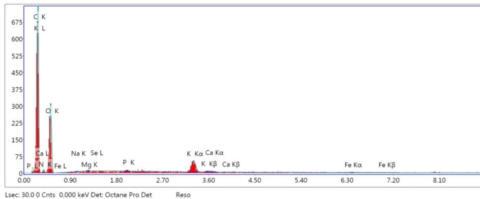
Fig. 2. Energy dispersive X-ray analysis (EDXA) of C1, C2, C3 and Control.
