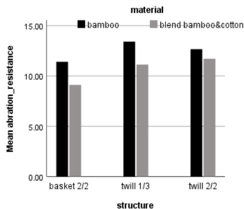
Fig. 9. Effect of material and structure on abrasion resistance (Loss of thickness).
