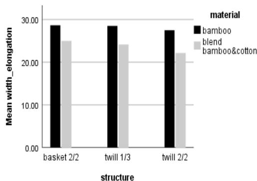
Fig. 8. Effect of material and structure on weft elongation (%).
