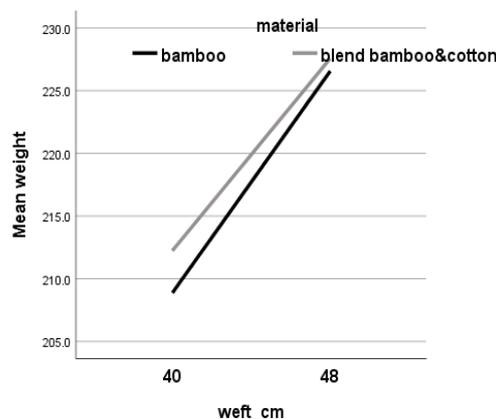
Fig. 10. Effect of Weft set on Weight (gm/m<sup>2</sup>).
