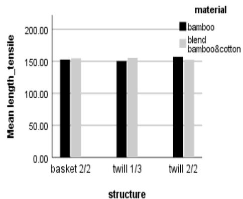
Fig. 5. Effect of material and structure on warp tensile strength (kg).
