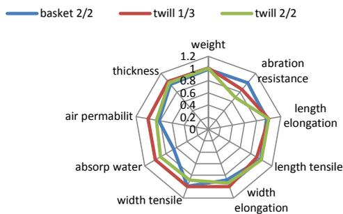
Fig. 20. Shows the radar charts of the bamboo 100% using 40 weft / cm.
