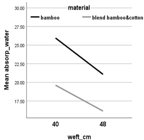
Fig. 13. Effect of Weft set on water absorb (%).
