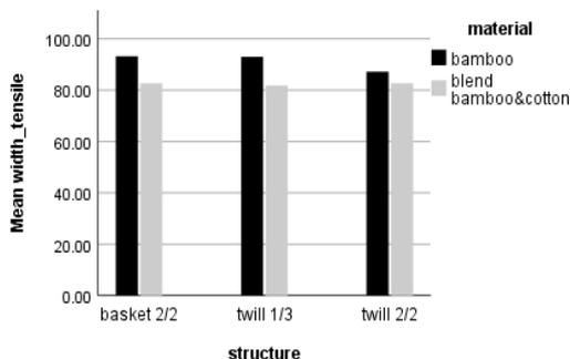
Fig. 7. Effect of material and structure on weft tensile strength (kg).
