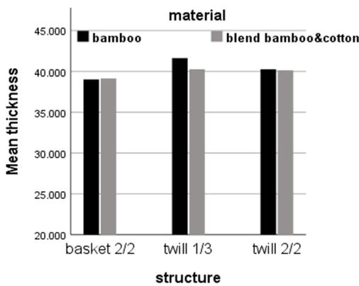
Fig. 2. Effect of material and structure on thickness (mm).
