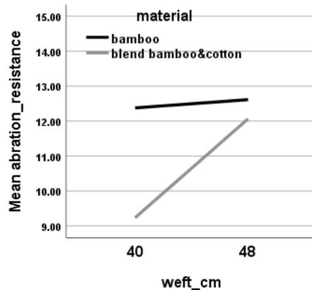
Fig. 18. Effect of Weft set on abrasion resistance (Loss of thickness %).
