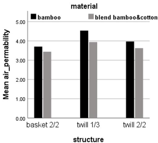
Fig. 3. Effect of material and structure on air permeability (cm<sup>3</sup>/cm<sup>2</sup>/sec).
