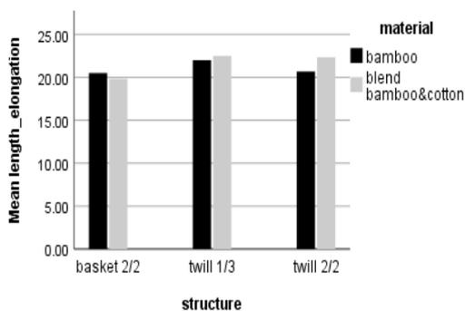
Fig. 6. Effect of material and structure on warp elongation (%).
