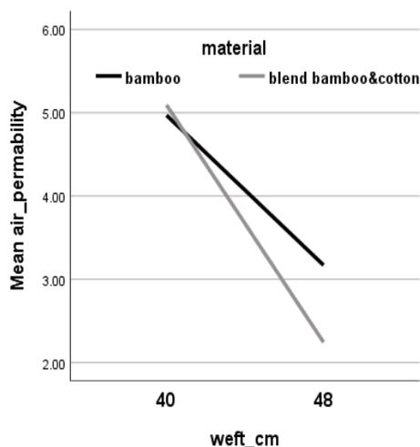
Fig. 12. Effect of Weft set on air permeability (cm<sup>3</sup>/cm<sup>2</sup>/sec).
