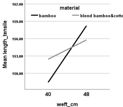
Fig. 16. Effect of Weft set on tensile strength of warp (kg).
