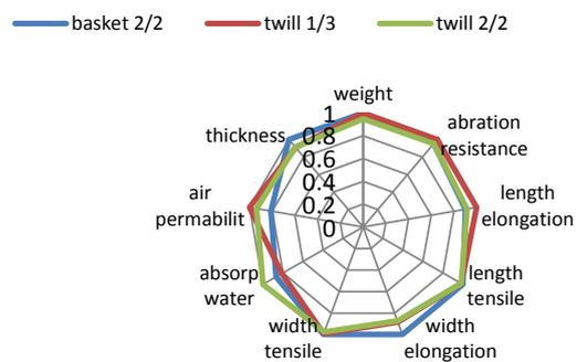
Fig. 19. Shows the radar charts of the bamboo 100% using 48 weft / cm.
