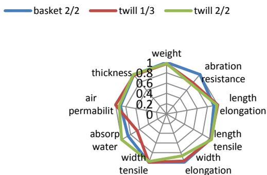
Fig. 22. Shows the radar charts of the blend bamboo using 40 weft / cm.
