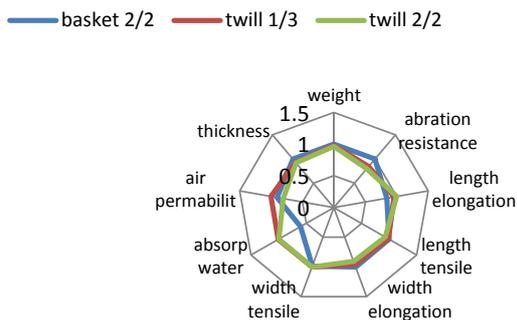
Fig. 21. Shows the radar charts of the blend bamboo using 48 weft / cm.
