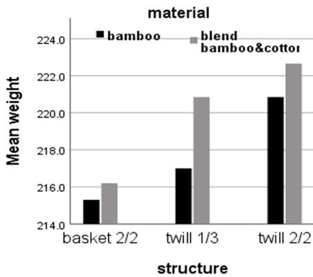
Fig. 1. Effect of material and structure on weight (gm/m<sup>2</sup>).
