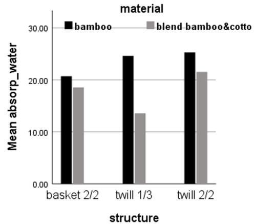
Fig. 4. Effect of material and structure on absorb water (%).
