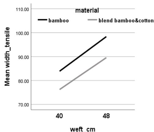
Fig. 14. Effect of Weft set on tensile strength of weft (kg).
