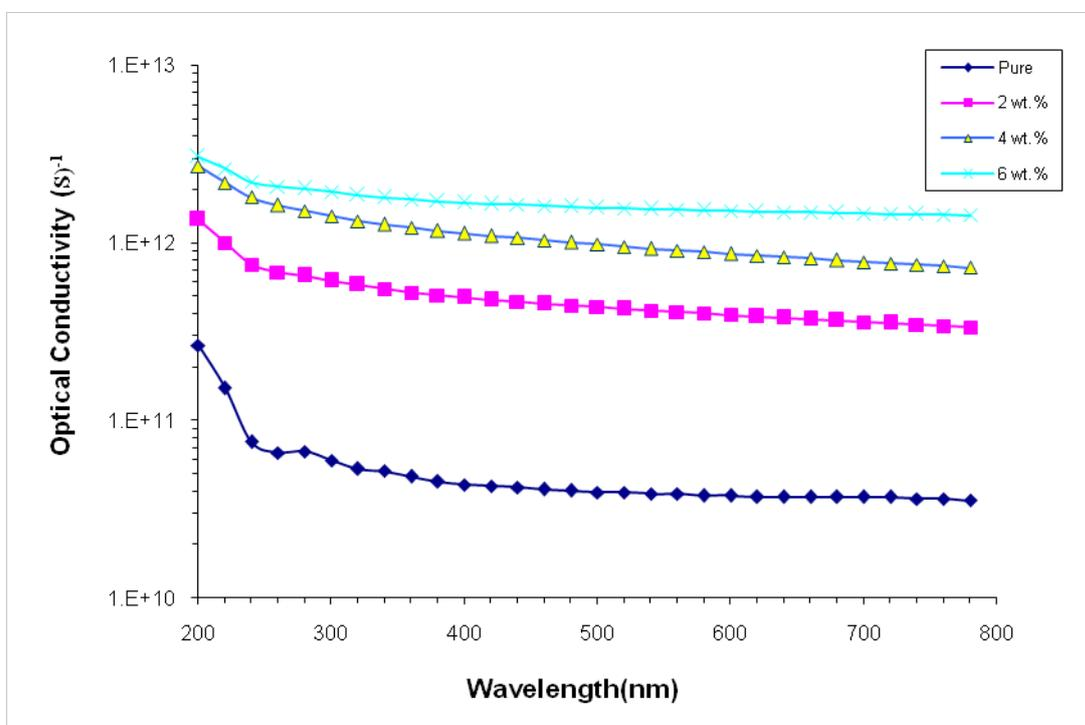
Fig. 9. Variation of optical conductivity for PVA/SiO<sub>2</sub> nanocomposites with photon energy.
