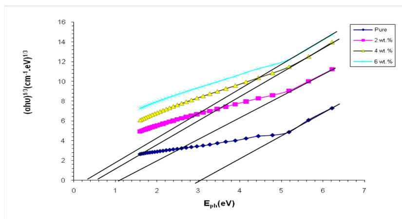
Fig. 4. Energies gaps for forbidden indirect transition of PVA/SiO<sub>2</sub> nanocomposites.
