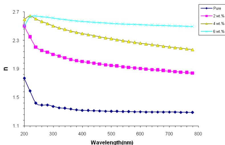
Fig. 6. Variation of refractive index with photon wavelength for (PVA-SiO<sub>2</sub>) nanocomposites.
