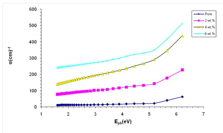
**Fig. 2.** Effect of silicon dioxide nanoparticles concentrations on the absorption coefficient of PVA .
