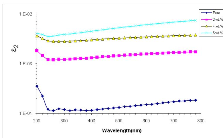
Fig. 7. variation of real part of dielectric constant for PVA/SiO<sub>2</sub> nanocomposites with photon wavelength.
