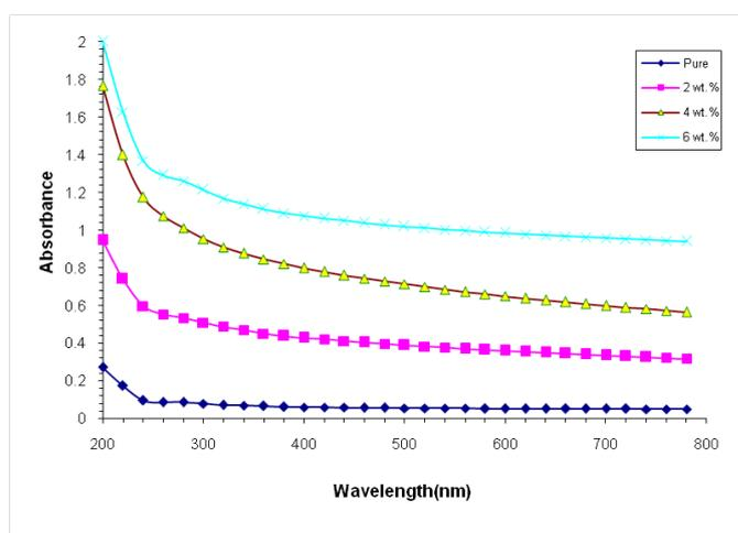
**Fig. 1.** Variation of optical absorbance of nanocomposites as function of wavelength for different silicon dioxide concentrations.
