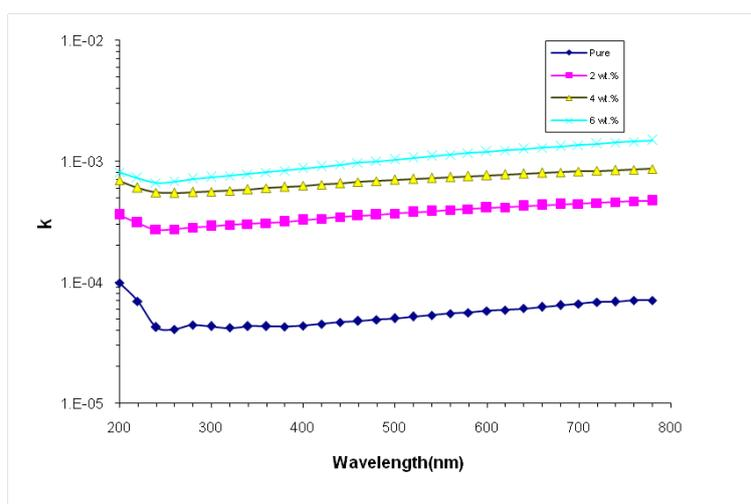
Fig. 5. Variation of the extinction coefficient with the incident photon wavelength of (PVA-SiO<sub>2</sub>) nanocomposites.
