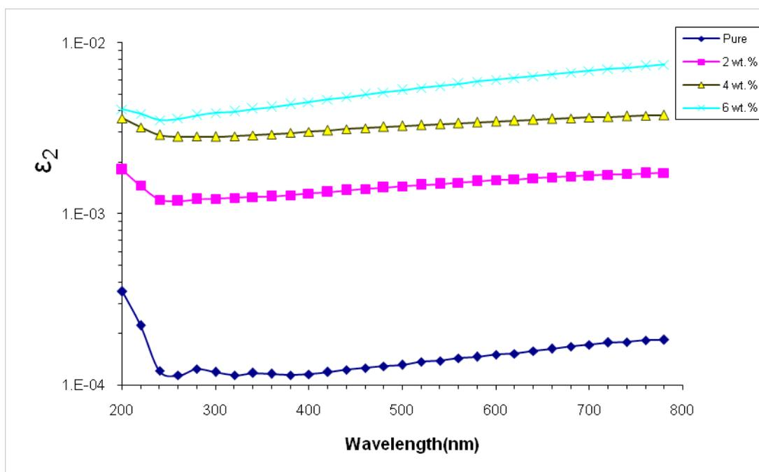
Fig. 8. Variation of imaginary part of dielectric constant for PVA/SiO<sub>2</sub> nanocomposites with photon wavelength.
