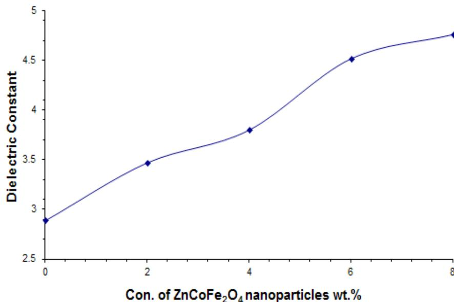
Fig. 3. The variation of dielectric constant for (PS-Cr<sub>2</sub>O<sub>3</sub>) nanocomposites with ZnCoFe<sub>2</sub>O<sub>4</sub> nanoparticles content at 100Hz.
