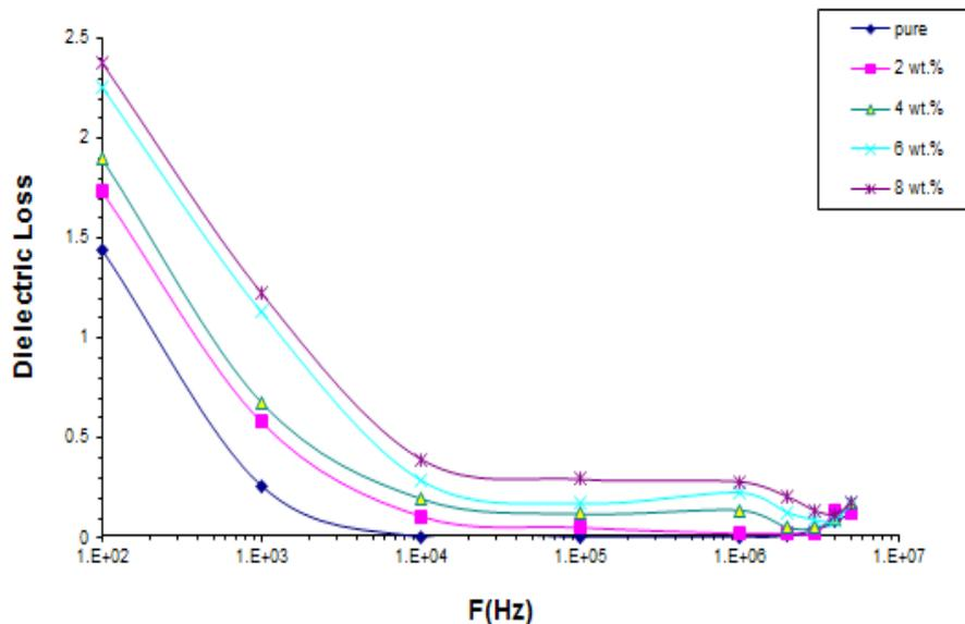
Fig. 2. The variation of dielectric loss with the frequency at room temperature.
