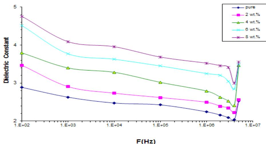
Fig. 1. The variation of dielectric constant with the frequency at room temperature.
