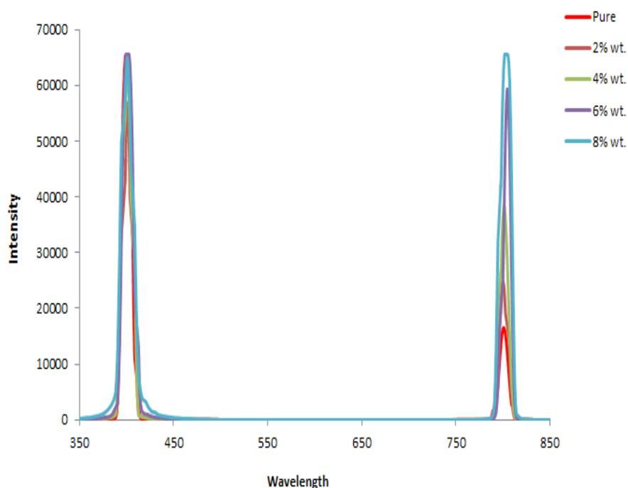
Fig. 7. The Fluorescent spectra of (PS-Cr<sub>2</sub>O<sub>3</sub>/ZnCoFe<sub>2</sub>O<sub>4</sub>) nanocomposites.
