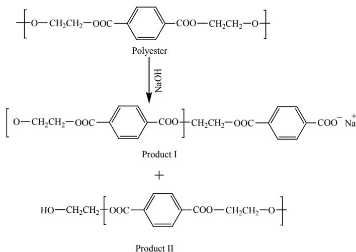
**Fig.1: Hydrolysis of polyester fabrics using sodium hydroxide product I and II: active hydrolyzed polyester fabrics**
