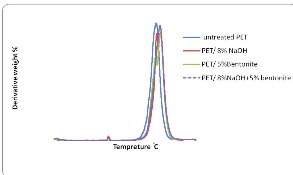
Fig. 6 (b):DTGA diagram of PET, PET/ 8% NaOH, PET/ 5%BNPs and PET/ 8%NaOH/ 5%BNPs.
