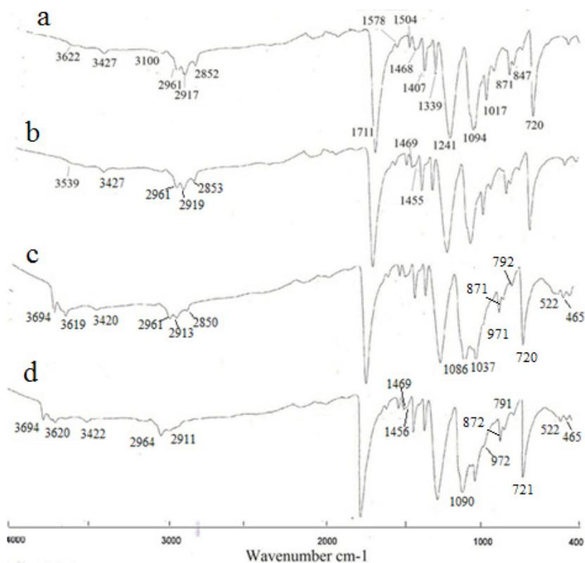
**Fig. 5.** FTIR spectra of (a) untreated PET, (b) PET/ 8%NaOH, (c) PET/ 5% Bentonite and (d) PET/ 8%NaOH/ 5% Bentonite.
