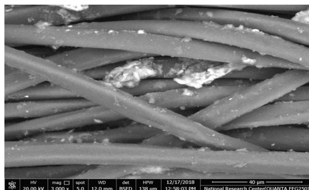
**Fig. 3 (b):** Treated sample with 8% sodium hydroxide followed by 5% BNPs by IR service technique
