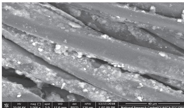
**Fig. 3 (c):** Treated sample with 8% sodium hydroxide followed by 5% BNPs by Pad dry cure technique.
