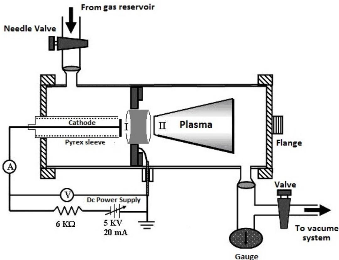
Fig. 1. The schematic diagram of DC pseudo plasma discharge device [5].
