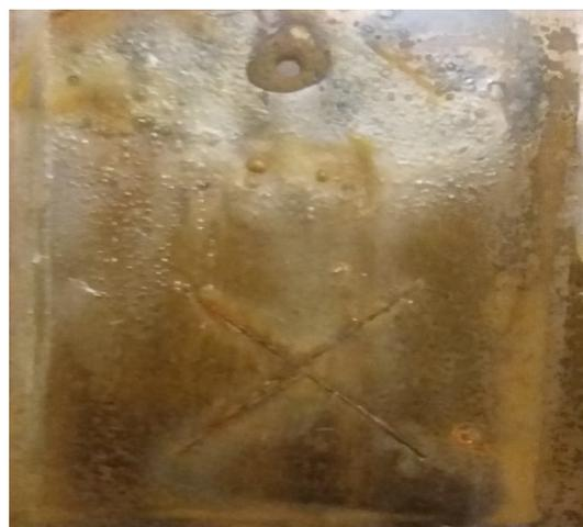
**F1.5****Fig. 6.** Corrosion test of steel panels under the coated films.
