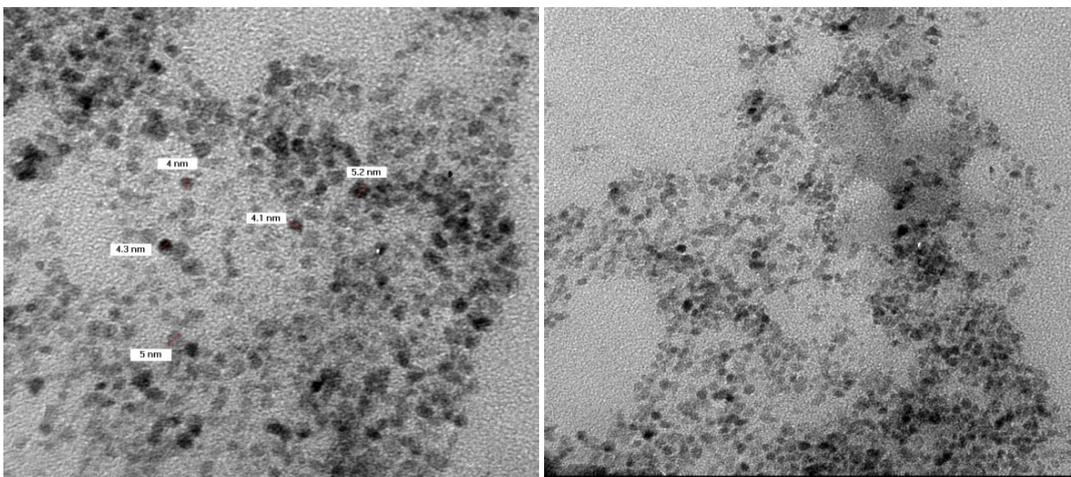
Fig. 3. HRTEM of NS particles.
