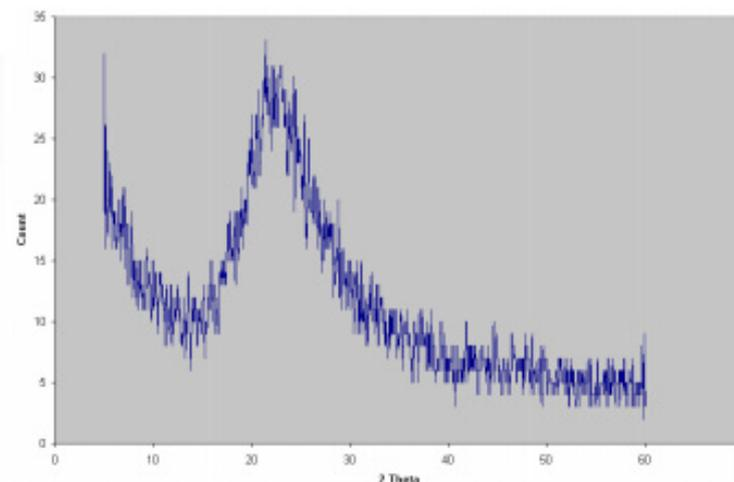
Fig. 4. XRD diffraction pattern of NS particles.
