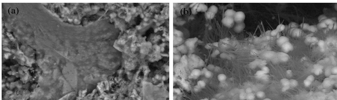
**Fig. 10. (a) micrograph of well dispersed CNTs, and (b) micrograph of agglomerated CNTs and NS particles.**
