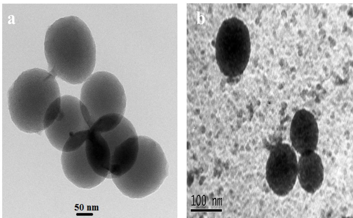
**Fig. 1.** TEM images of (a) mesoporous silica nanoparticles (MSNPs) and (b) curcumin loaded mesoporous silica nanoparticles (Cur-MSNPs). The scale bars of a & b are 50, 100 nm respectively.
