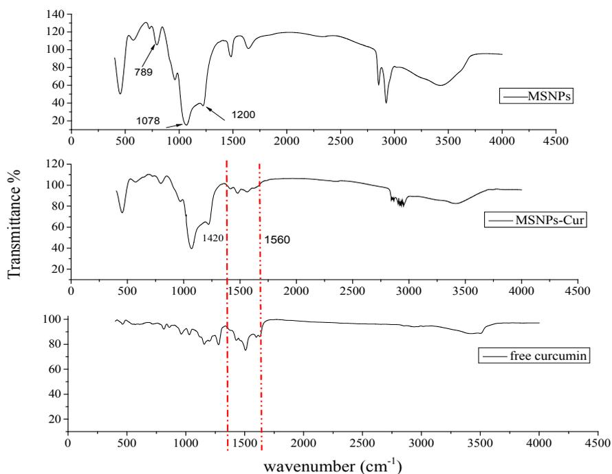
Fig. 3. FTIR spectra for: mesoporous silica nanoparticles (MSNPs), curcumin-loaded mesoporous silica nanoparticles (Cur-MSNPs) and free curcumin.
