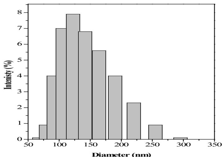
Fig. 2. Particle size distribution of MSNPs.
