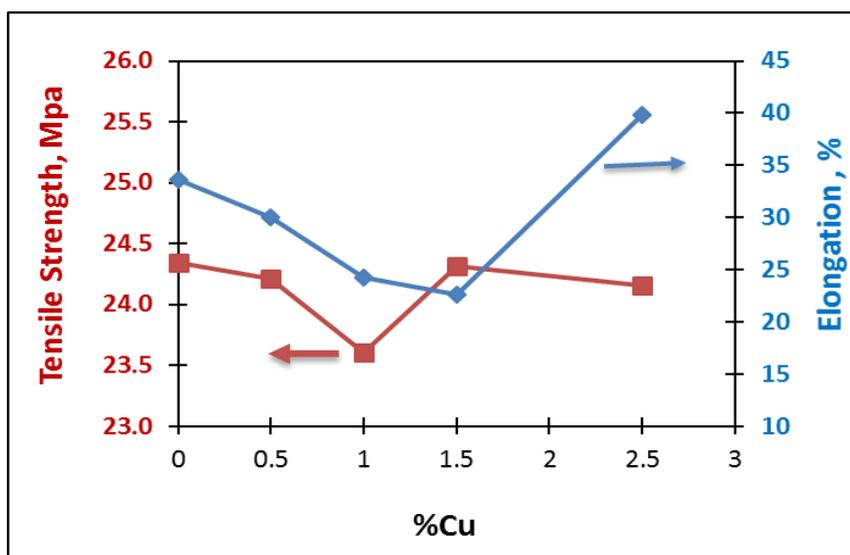
Fig. 8. The tensile strength and elongation variation for PP/nano-copper composite materials.
