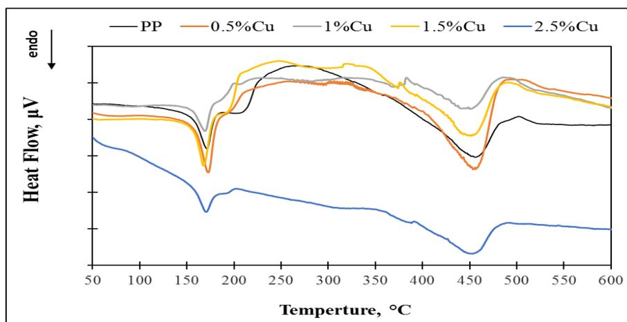
Fig. 7. Thermal analysis PP and PP/nano-copper composite materials.
