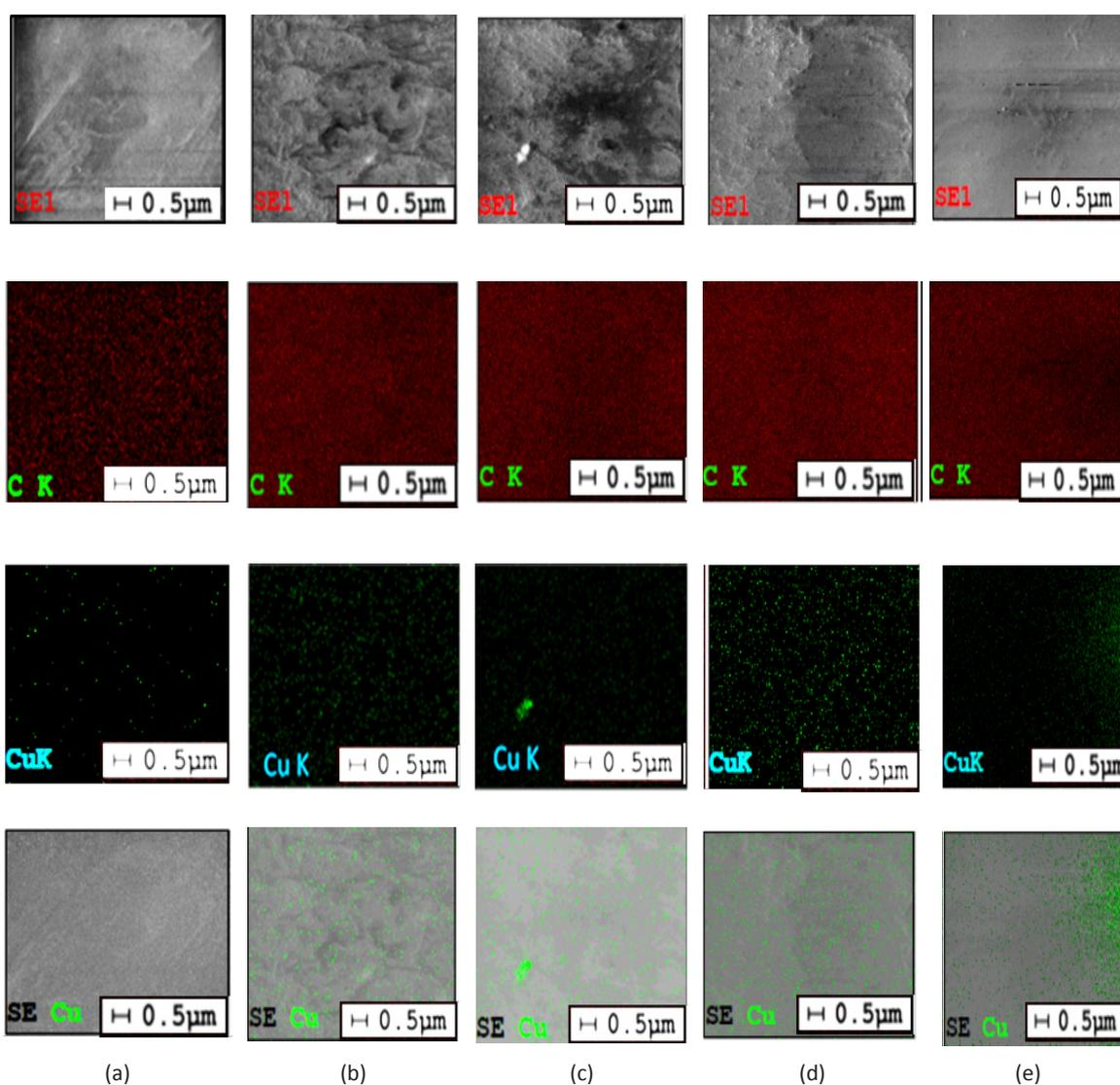
Fig. 4. The EDAX mapping of the PP/Nano-Copper composite for (a) 0.5 wt%Cu, (b) 1 wt%Cu, (c) 1.5 wt%Cu, (d) 2 wt%Cu and (e) 2.5 wt%Cu.
