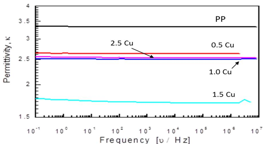
Fig. 5. The dielectric permittivity of PP and PP/nano-copper composite materials.
