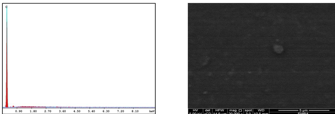
Fig. 3. the SEM and EDAX of pure PP.
