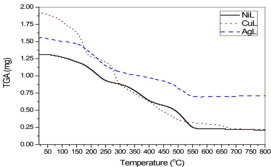
Fig. 3. Thermal analysis (TG) of Ni (1), Cu (2) and Ag (4) complexes.
