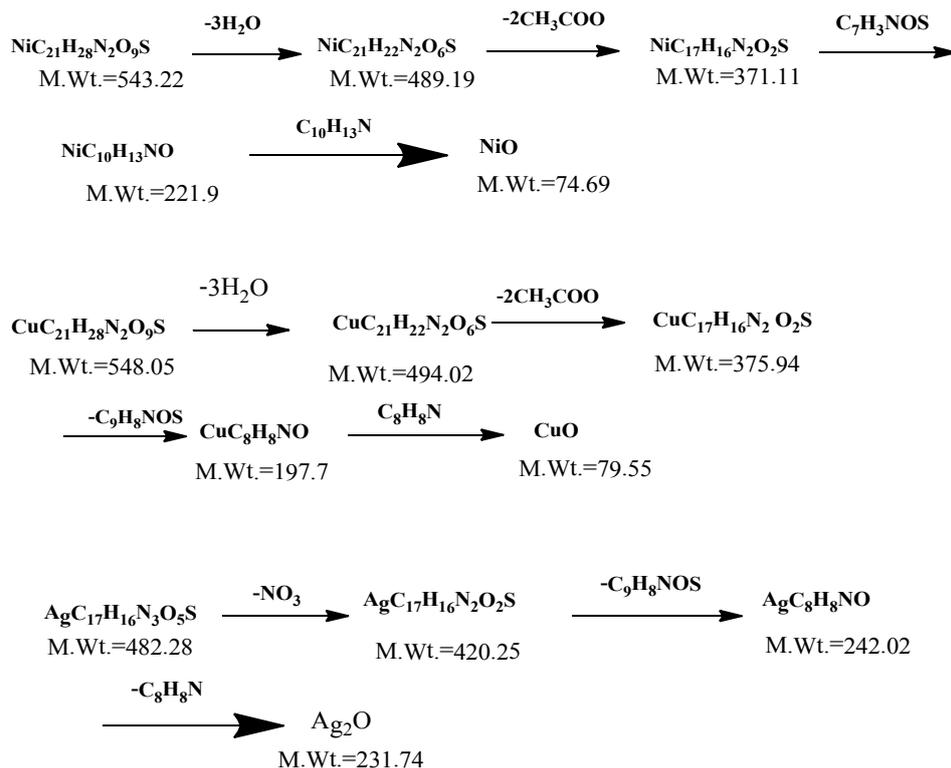
Scheme 3. Thermal decomposition of metal complexes (1, 2 and 4)
