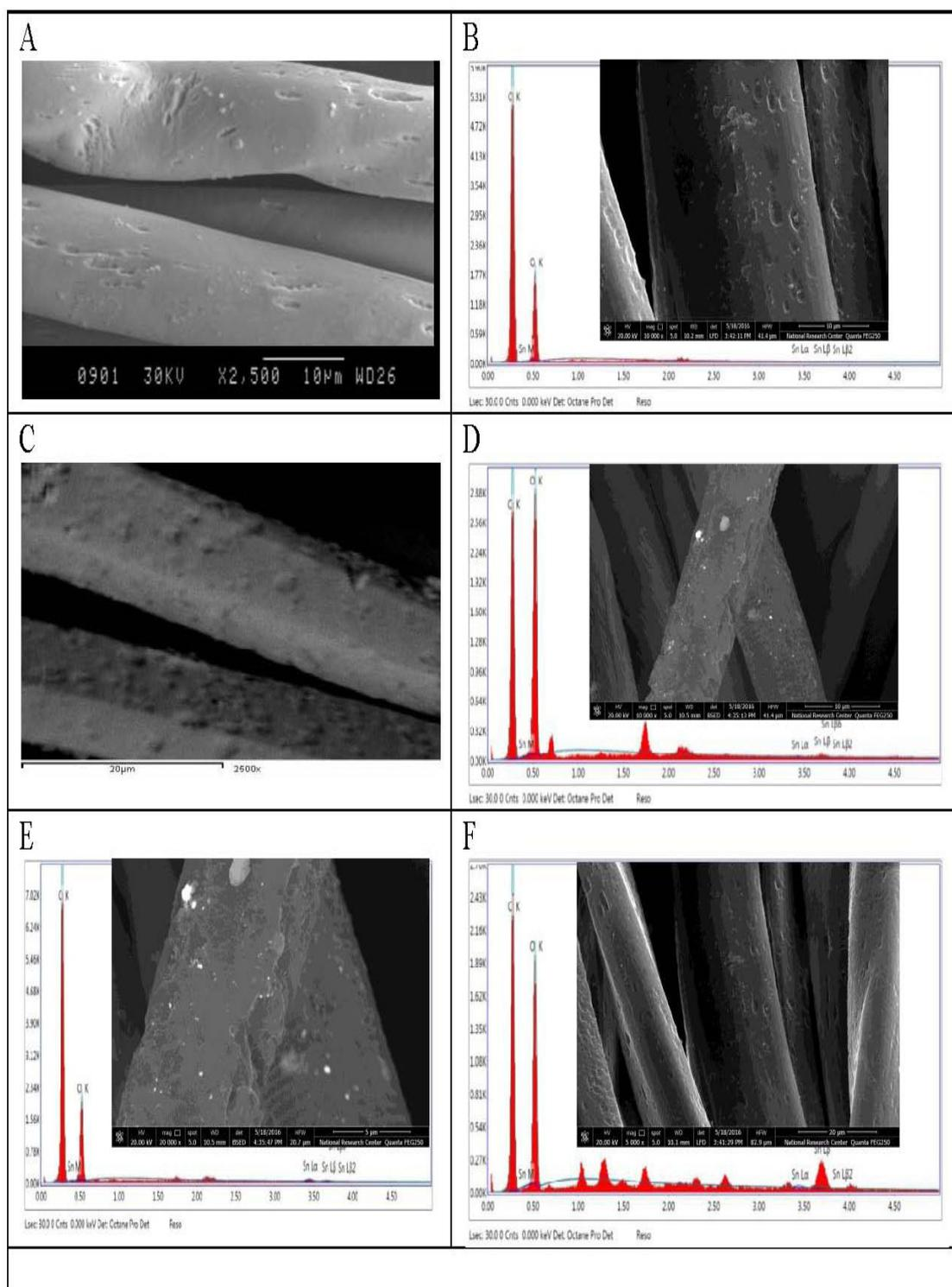
**Fig. 3.** SEM and EDX micrographs of bleached and partially hydrolyzed PET fabrics loaded with  $\text{SnO}_2$  NPs\* (X2000).
