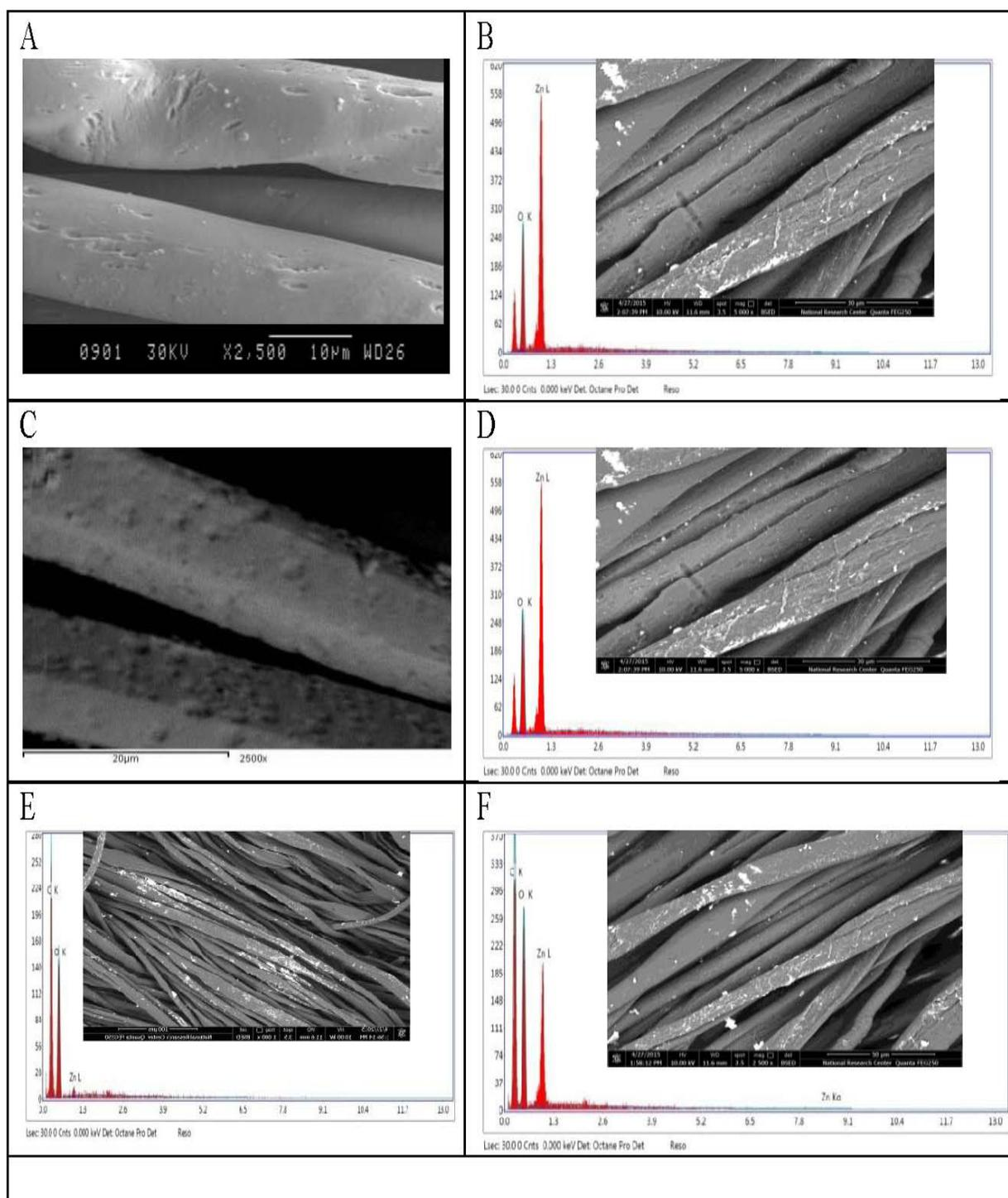
**Fig. 2. SEM and EDX micrographs of bleached and partially hydrolyzed PET fabrics loaded with ZnO NPs\* (X2000).**
