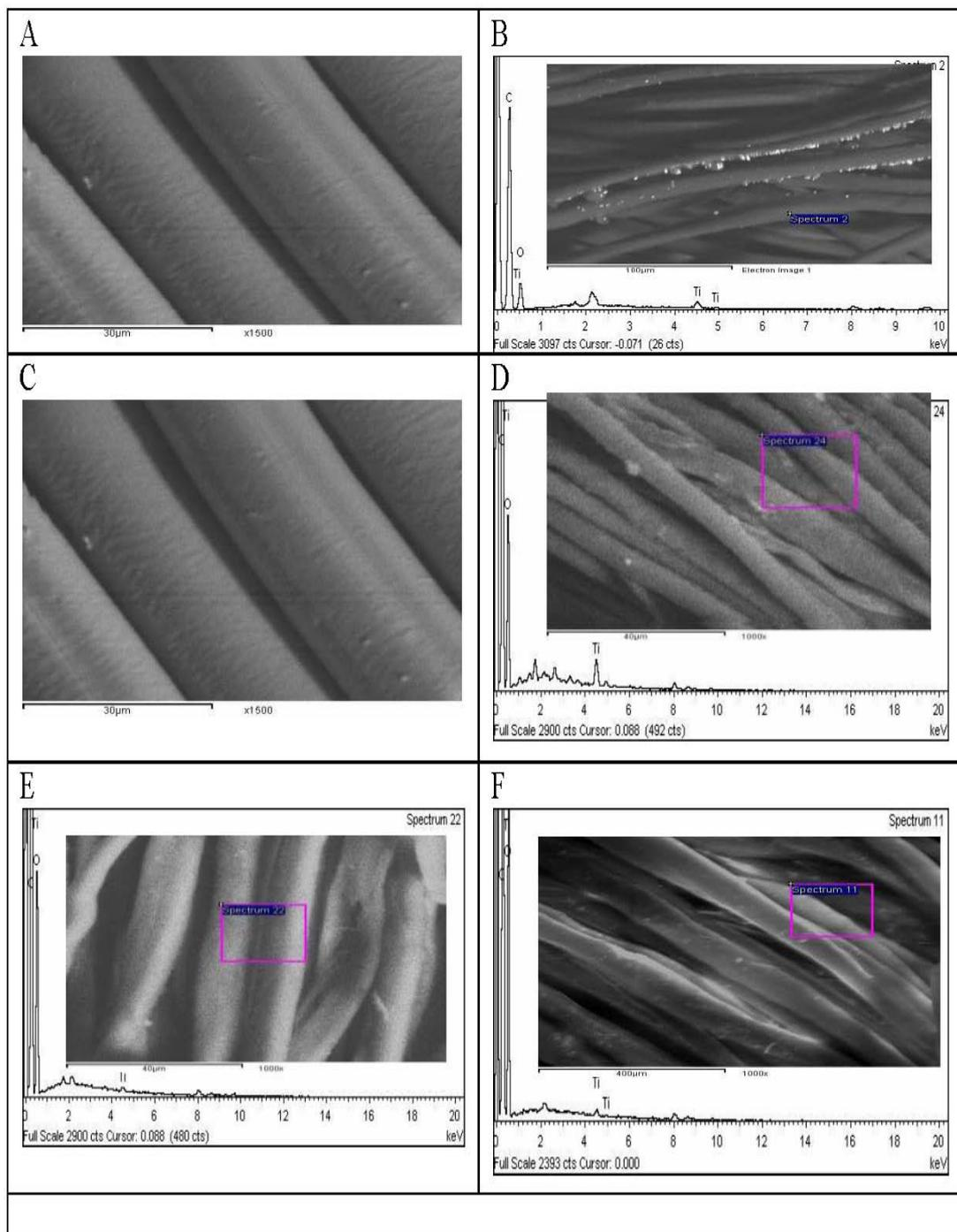
**Fig. 1. SEM and EDX micrographs of bleached and partially hydrolyzed PET fabrics loaded with  $\text{TiO}_2$  NPs\* (X2000).**
