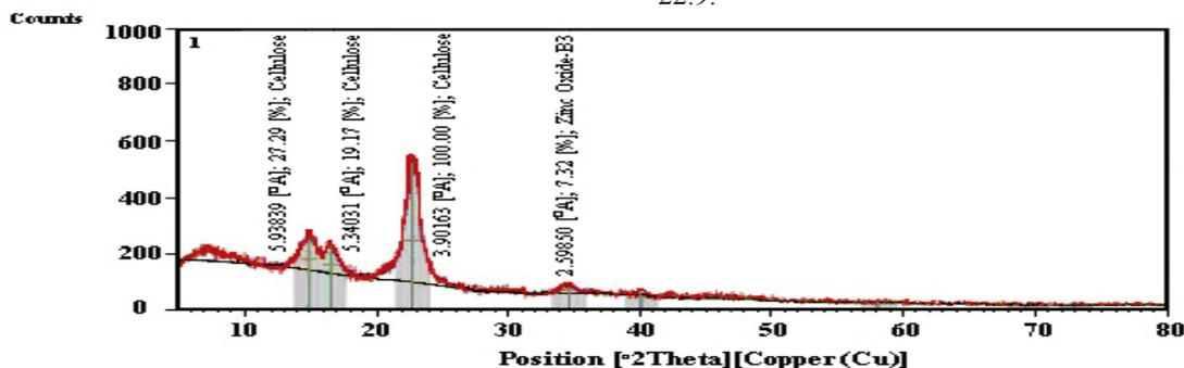
Fig. 5. XRD of CMC fabric treated with nano zinc oxide
