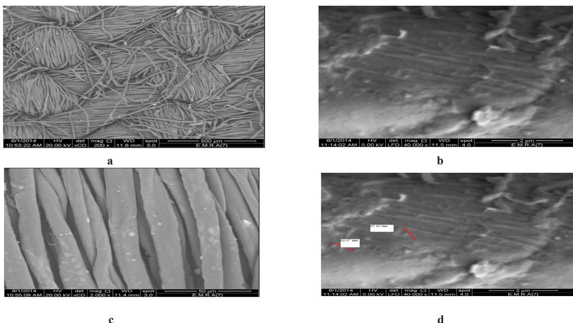
**Fig. 3.** SEM image of surface morphology of untreated cotton fabric (a-c), and carboxymethylated cotton fabric (d)
