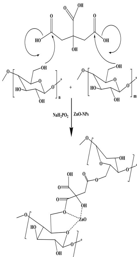
**Fig. 6. Scheme mechanism between CMC with citric acid and nano zinc oxide**
