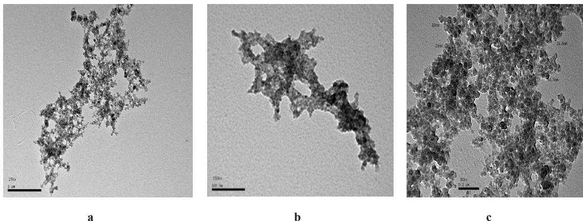
**Fig. 2 (a-c).** TEM image of nano zinc oxide particle with different particle size a; 19nm, b; 30nm, and c; with 40.5nm
