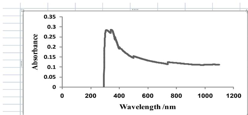
Fig. 4. UV-Visible curve of nano zinc oxide.
