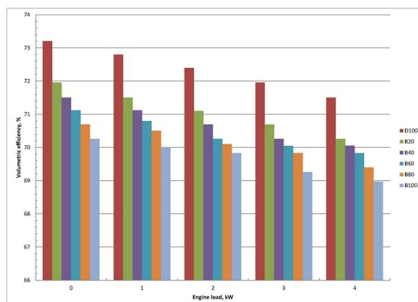
**Fig. 6.** Effect of engine load and percentage of catalytically cracked used cooking oil in its blend with diesel fuel on the volumetric ratio.
