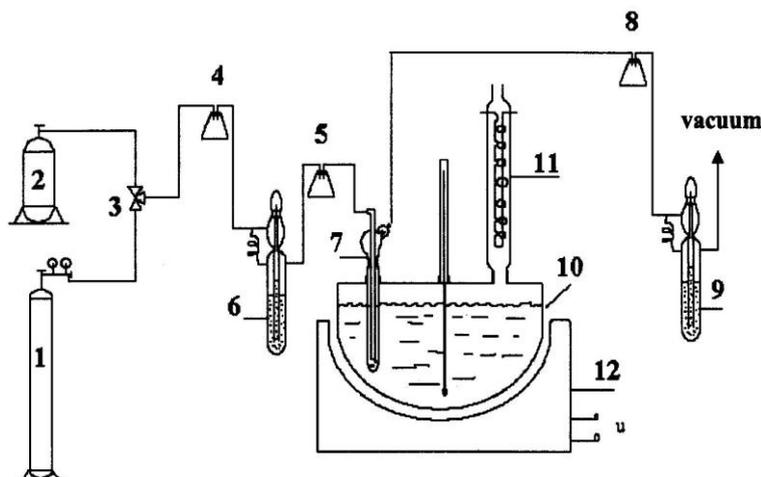
**Fig.1. Apparatus of the hydroxyethylation (1.N<sub>2</sub>,2. ethylene oxide, 3. valve, 4,5,8. buffers, 6,9. differential manometers, 7. semimicro reactor, 10. boiling bath, 11. cooler, 12. heater).**
