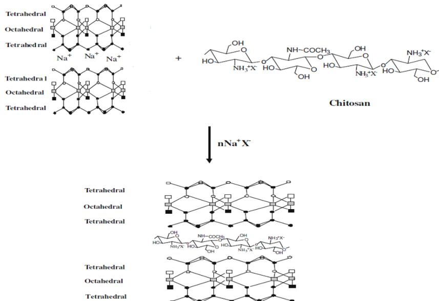
**Fig. 2. Schematic illustration of intercalation of chitosan in the interlayer space between the MMT clay.**
