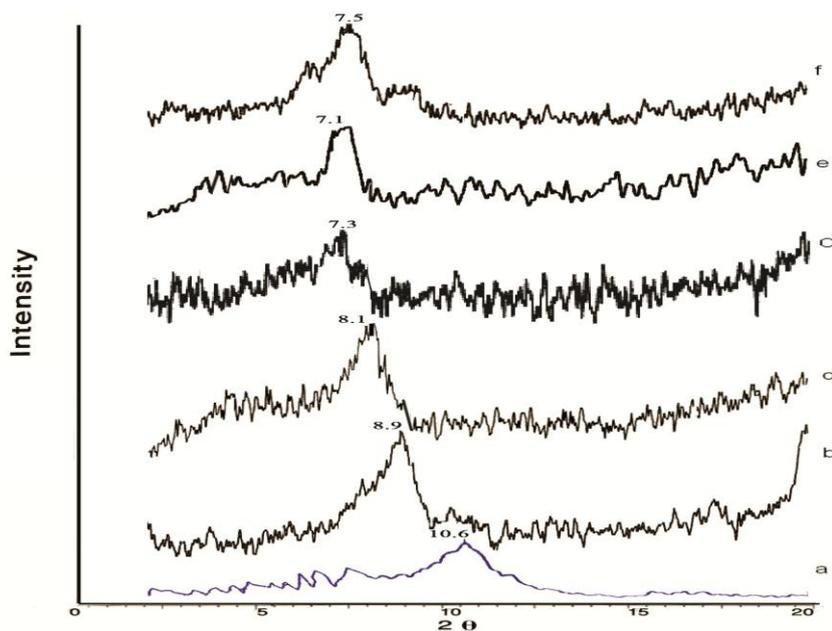
Fig. 5. X-ray diffraction patterns for (a) neat MMT, MMT modified by chitosan at temperatures of (b) 30 °C, (c) 40 °C, (d) 50 °C, (e) 60 °C and (f) 70 °C.
