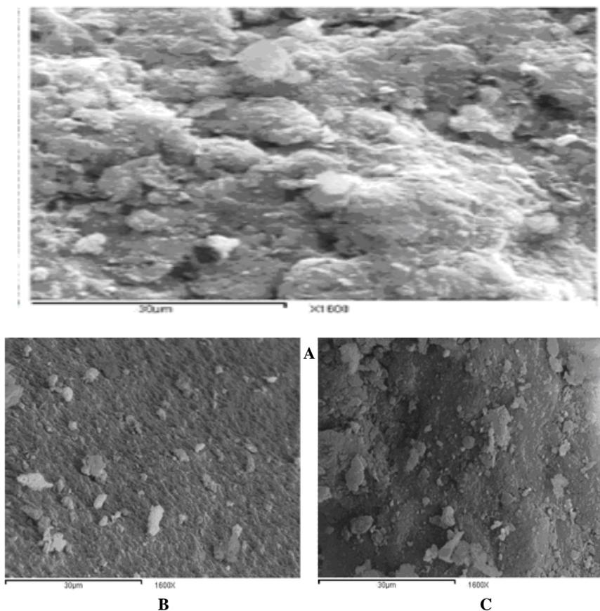
**Fig. 7 . SEM for A) pristine MMT clay, B) MMT clay modified by chitosan and C) MMT clay modified by aminated starch.**
