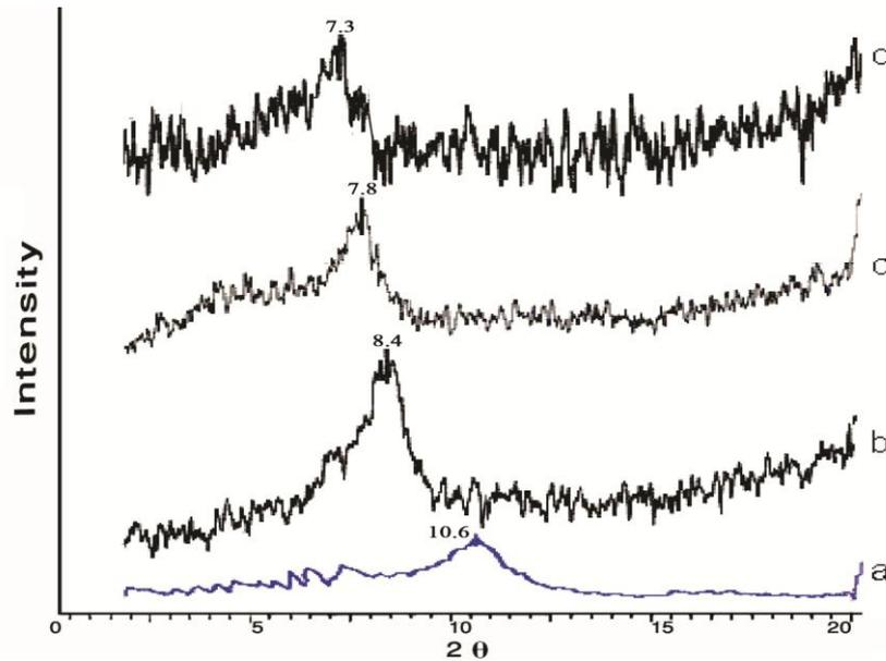
Fig. 3. X-ray diffraction patterns for (a) neat-MMT, MMT modified by chitosan at (CS/MMT) ratios of (b) 1:2, (c) 1:1, and (d) 2:1.
