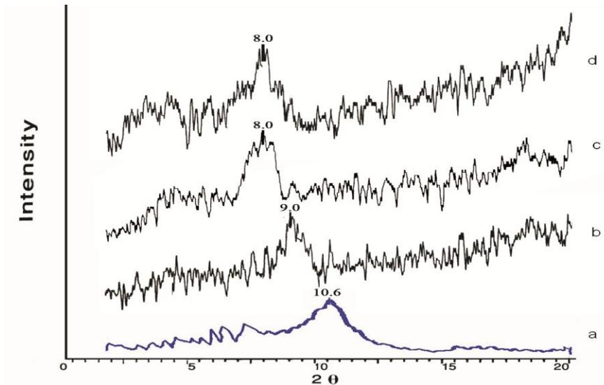
Fig. 4. X-ray diffraction patterns for (a) neat-MMT, MMT modified by aminated starch at (AmS/MMT) ratios of (b) 1:2, (c) 1:1, and (d) 2:1.
