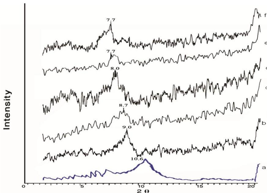
Fig. 6. X-ray diffraction patterns for (a) neat MMT, MMT modified by aminated starch at temperatures of (b) 30 °C, (c) 40 °C, (d) 50 °C, (e) 60 °C and (f) 70 °C.
