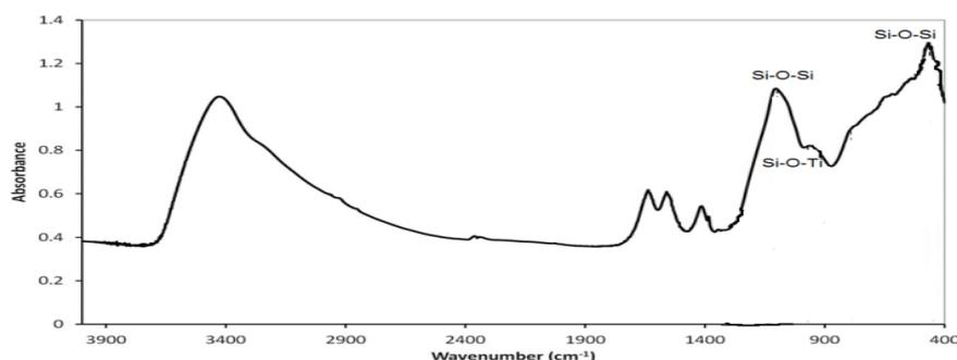
**Fig. 12.** FTIR spectrum of synthesized TiO<sub>2</sub>/SiO<sub>2</sub> 50:50 over 400–4000 cm<sup>-1</sup>.
