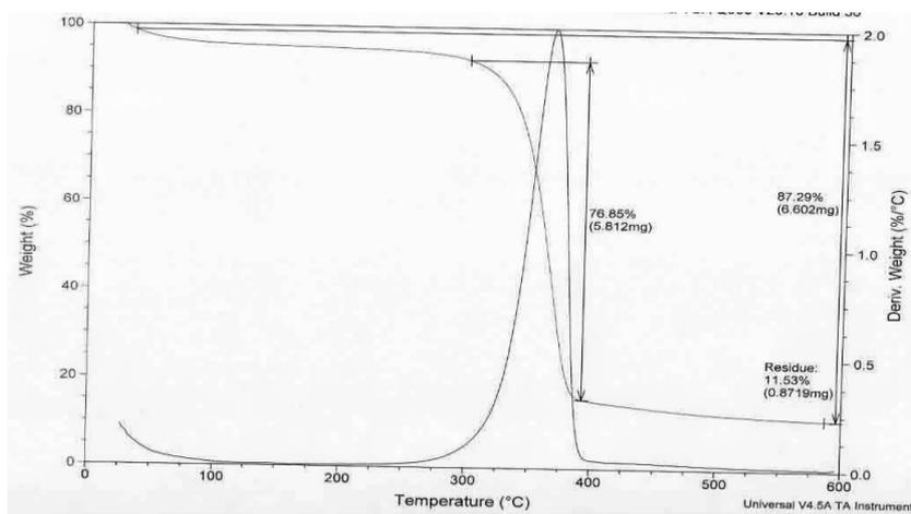
**Fig.7. TGA curve of untreated cotton fabric.**
