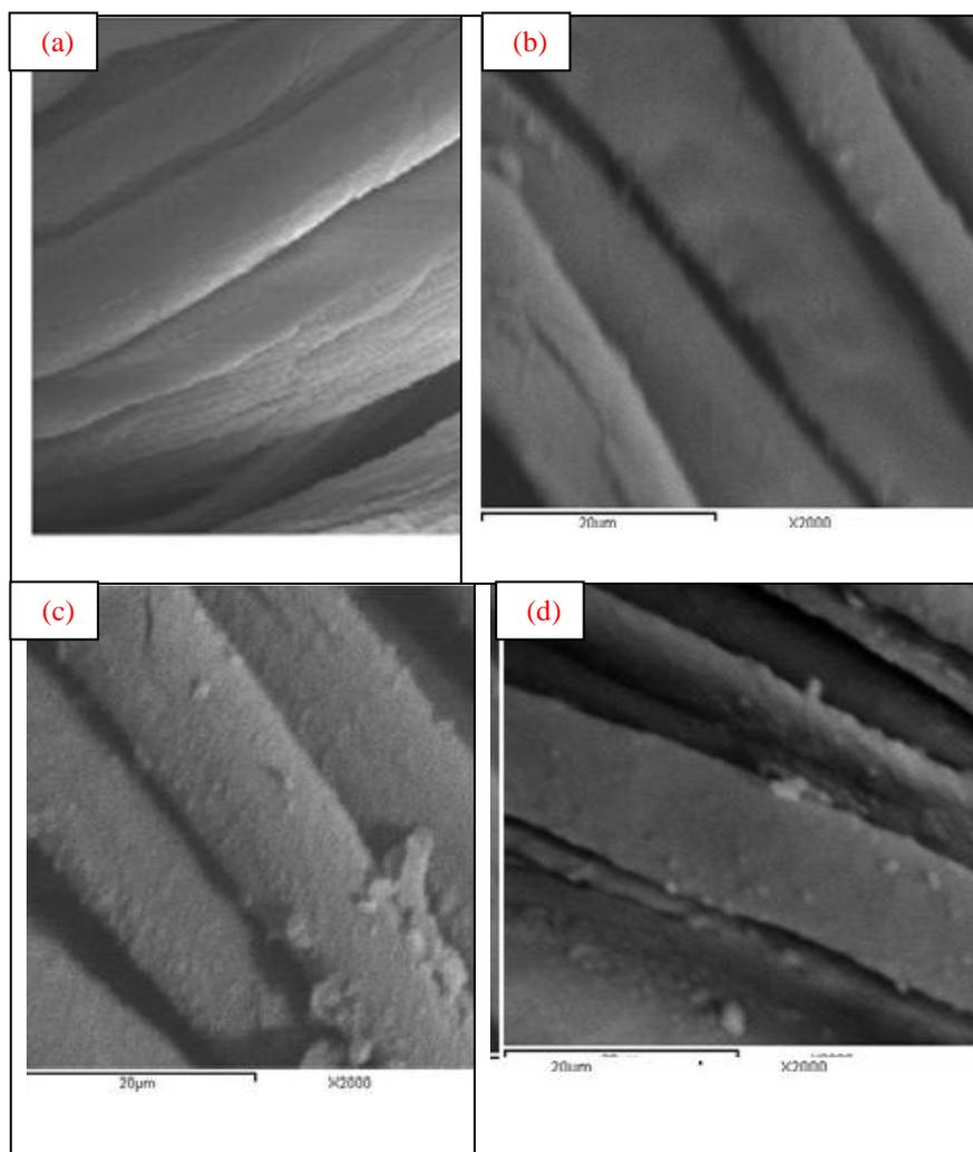
**Fig. 13.** SEM (a) untreated cotton fabric (b) cotton fabric treated with  $\text{TiO}_2$  nanoparticles (c) cotton fabric treated with  $\text{TiO}_2/\text{SiO}_2$  nanoparticles (d) superhydrophobic cotton fabric treated with  $\text{TiO}_2/\text{SiO}_2$  sol post treated with TOES/GPTMS.
