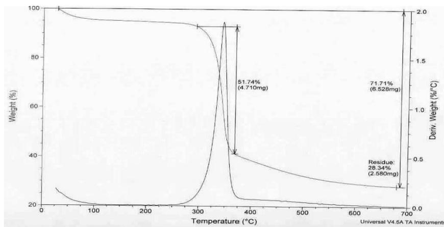
**Fig. 11.** TGA curve of cotton treated with TiO<sub>2</sub>/SiO<sub>2</sub> nanoparticles post treated with T/G Where TEOS/GPTMS.
