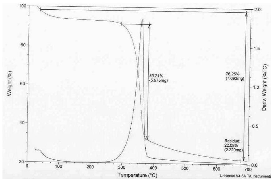
**Fig. 10.** TGA curve of cotton treated with TiO<sub>2</sub>/SiO<sub>2</sub> nanoparticles post treated with T TEOS.
