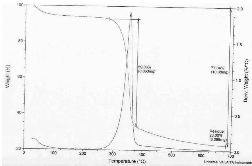
**Fig. 8. TGA curve of cotton treated with SiO<sub>2</sub> nanoparticles post treated with TEOS.**
