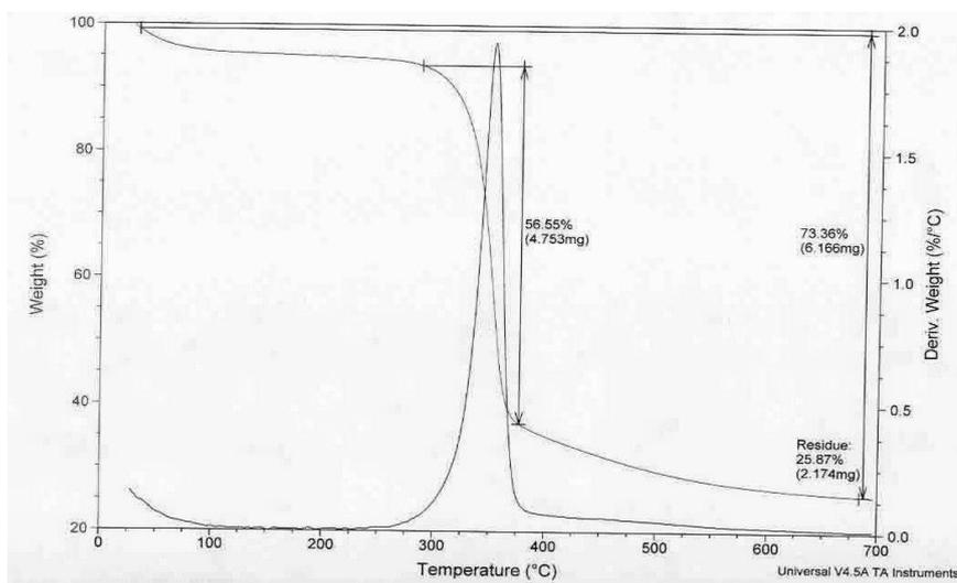
**Fig. 9.** TGA curve of cotton treated with SiO<sub>2</sub> nanoparticles post treated with T/G TEOS/GPTMS.
