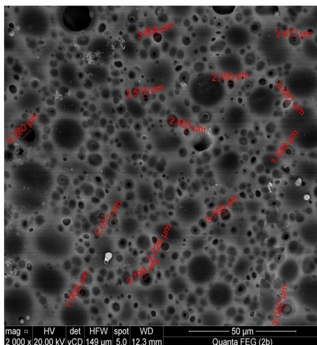
Fig. 2. SEM image of the prepared membrane without using additive.
