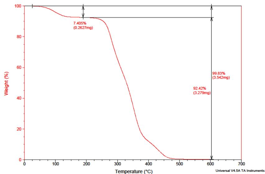
Fig. 5. DSC-TGA Curve of the prepared membrane without using PEG6000 .
