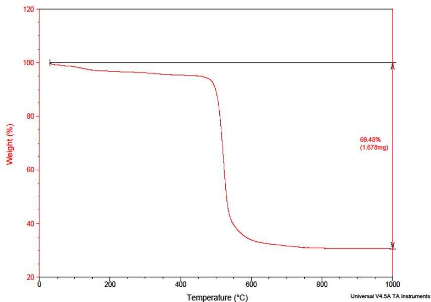
**Fig. 7. DSC-TGA Curve of the prepared membrane using 5wt% of PEG6000.**
