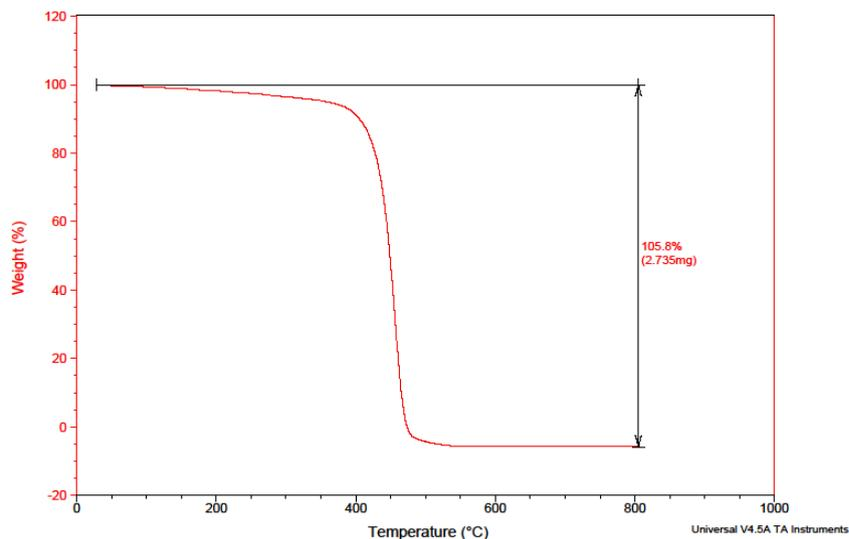
Fig. 6. DSC-TGA Curve of the prepared membrane using 4 wt% of PEG additive .
