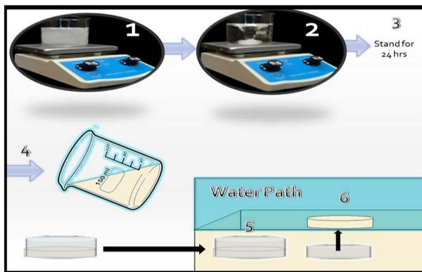
**Fig. 1. Graphical representation shows membrane preparation via phase inversion method.**
