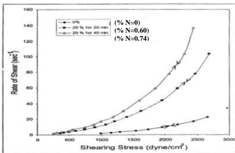
Fig. 2. Effect of urea concentration & reaction time on the apparent viscosity of carbamated fenugreek glactomannan gum (6%) at different rates of shear (after 24 hr storing).
