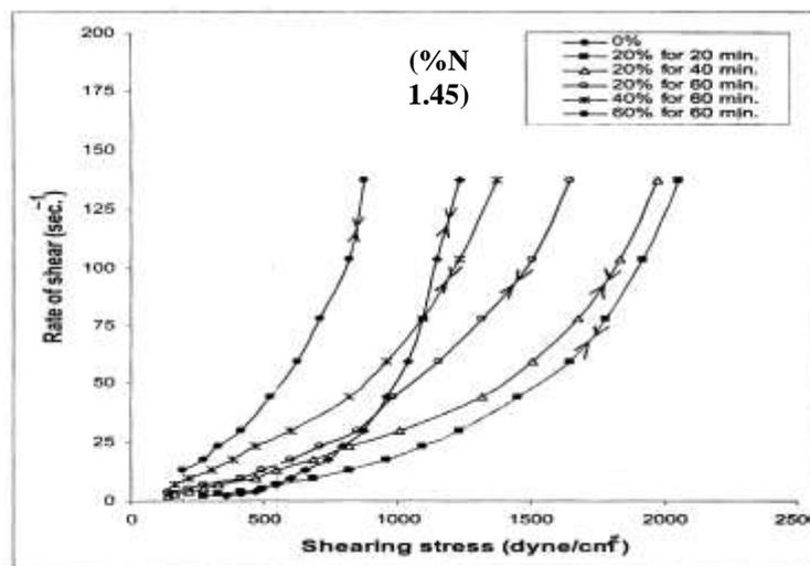
**Fig. 5.** Effect of urea concentration & reaction time on the apparent viscosity of carbamated fenugreek galactomannan gum (6%) treated with NaOH (1%) at different rates of shear (after 3 days. storing).
