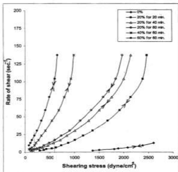
Fig. 3. Effect of urea concentration & reaction time on the apparent viscosity of carbamated fenugreek galactomannan gum (6%) at different rates of shear (freshly prepared).
