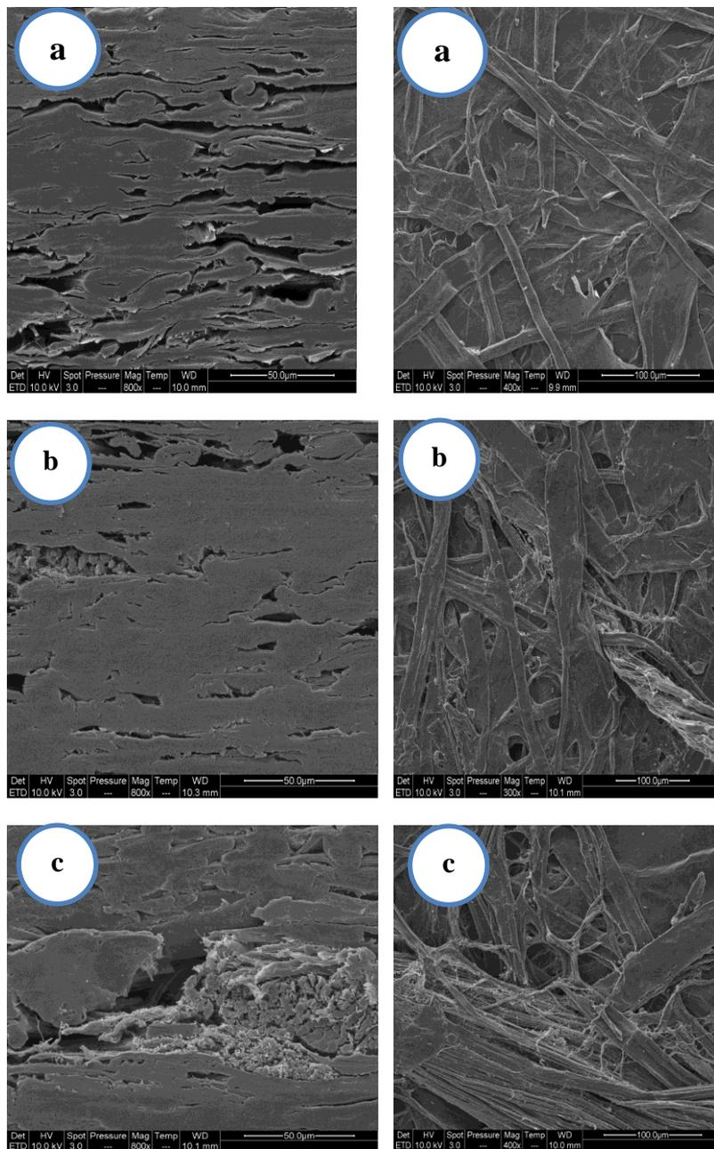
**Fig. 1c.** SEM images of a) blank carton sheet with fractural and surface image as well as carton sheet with different ratios of treated II, b) 6% and c) 12% with fractural and surface image.
