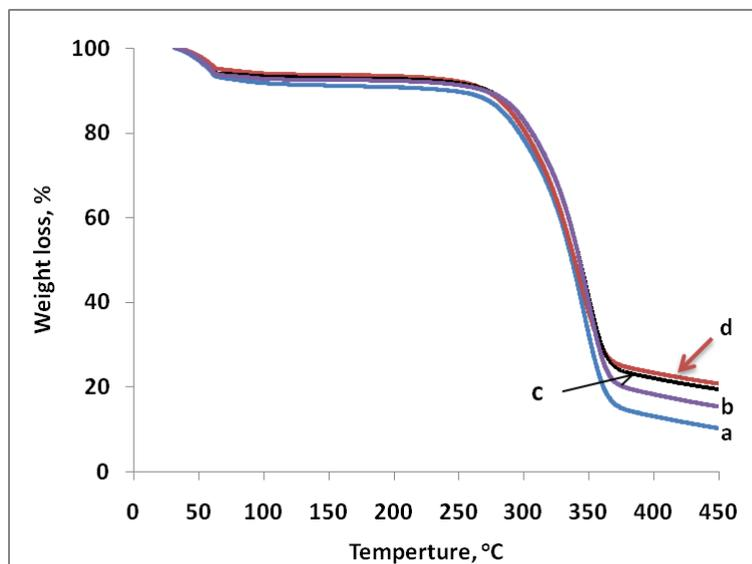
Fig. 2b. TGA of a) blank carton sheet as well as carton sheet with different ratios of treated I b)6 %, c) 9% and d) 12 %.
