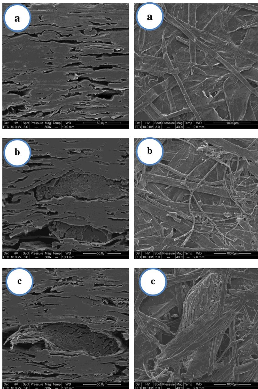
**Fig. 1b.** SEM images of a) blank carton sheet with fractural and surface image as well as carton sheet with different ratios of treated I, b) 6% and c) 12% with fractural and surface image.
