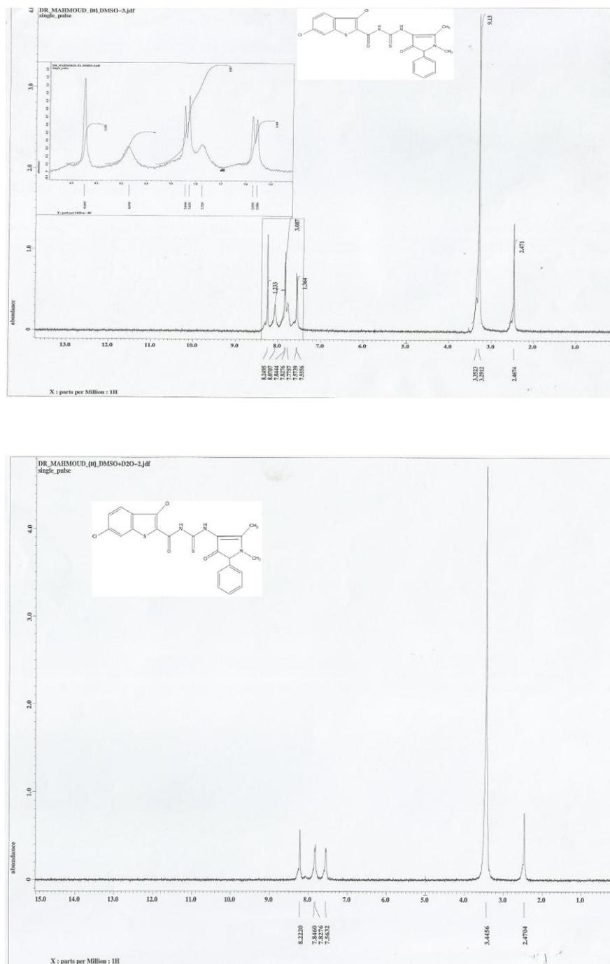
Fig. 6.  $^1\text{H}$ NMR spectrum of (II).
