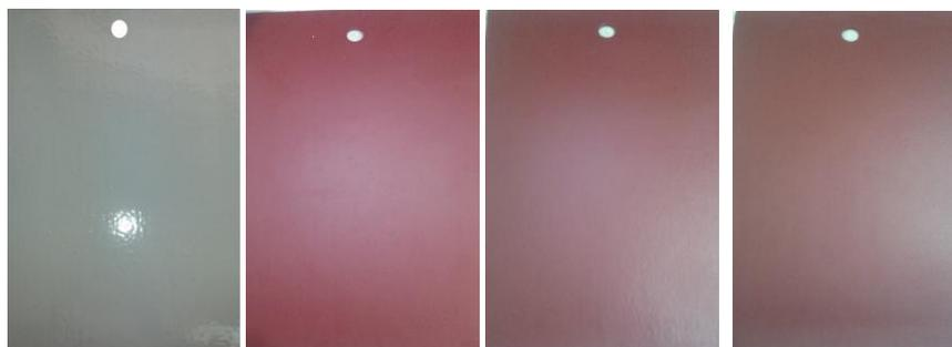
From the back face where no anti-fouling paint (epoxy coat only) (Blank sample) Compound (I) Compound (II) Compound (III)
