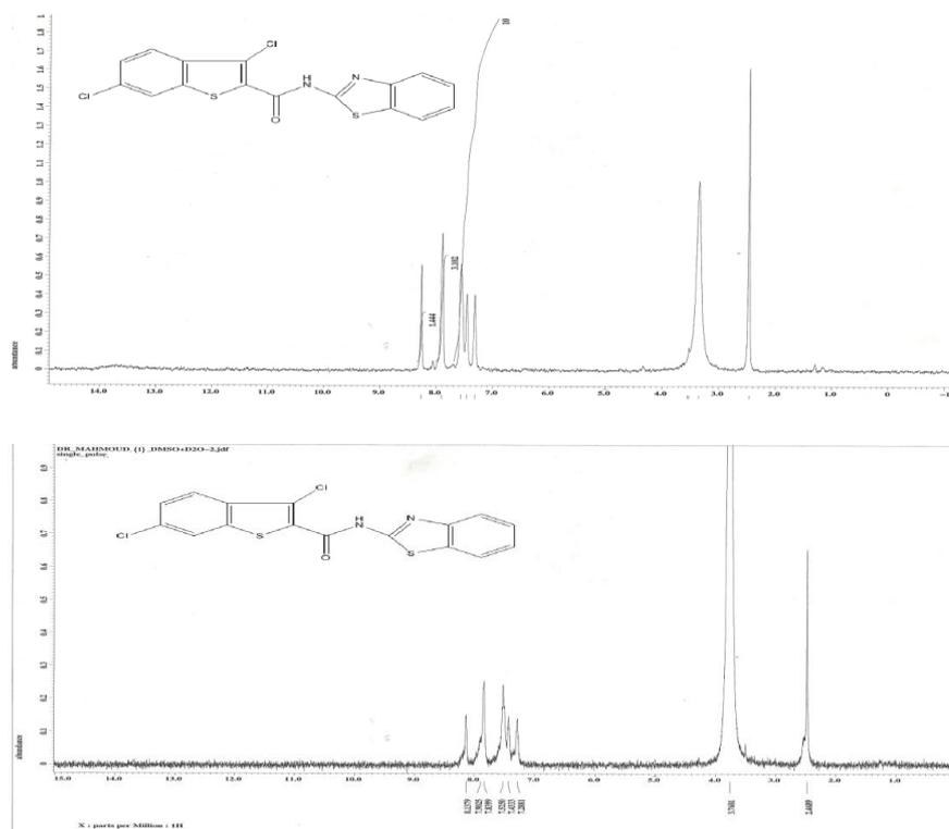
Fig. 3. <sup>1</sup>H NMR spectrum of (I).
