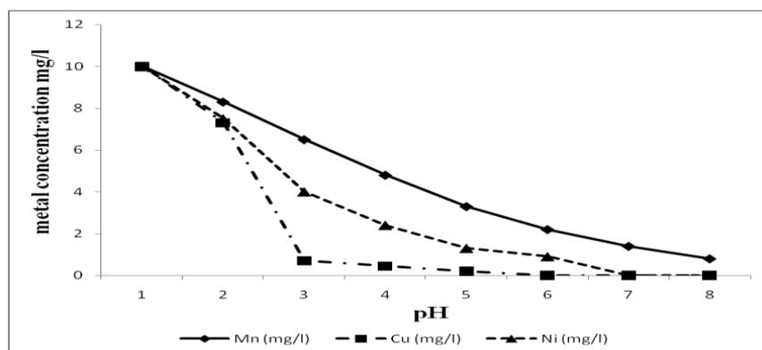
Fig. 5. Effect of different doses of lime (CaO) on the precipitation of Mn, Cu and Ni in artificial contaminated water.
