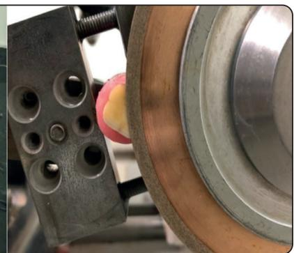
Fig. (3): flattening of occlusal surface
