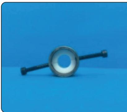
Fig. (1): Teflon mold with corresponding metal ring and paralleling screws (Top view)
