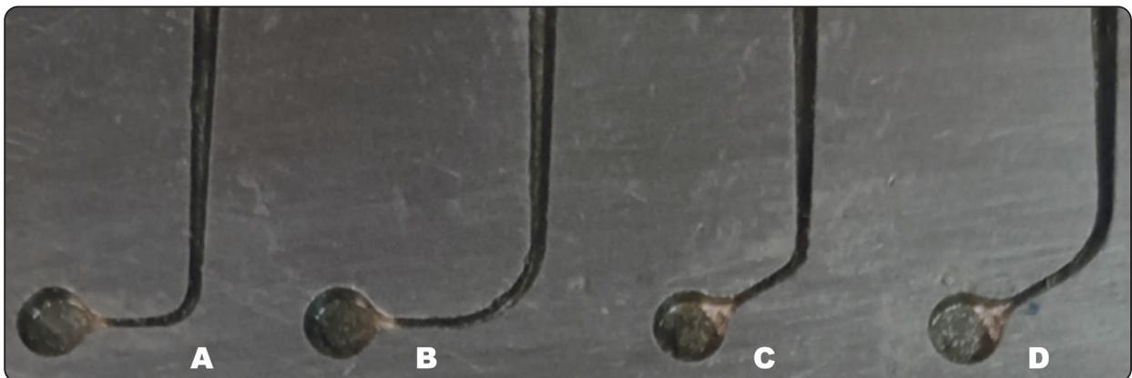
Fig. (1): Cyclic fatigue testing block; (a) angle 90° radius 2.5mm, (b) angle 90° radius 5mm, (c) angle 60° radius 2.5 mm, (d) angle 60° radius 5mm
