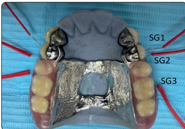
Fig. (6): Micro-strain gauges attached to the printed model with the channels' specification.
