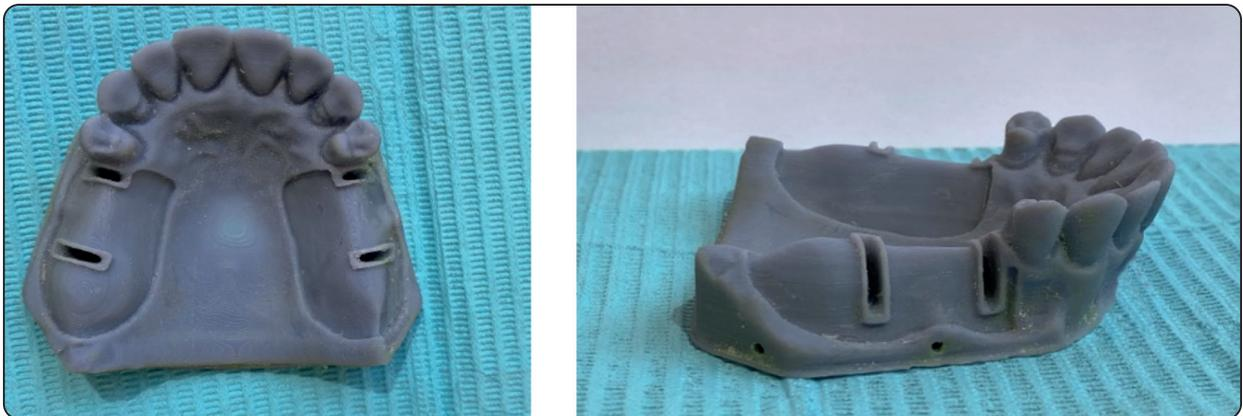
Fig. (2): The printed model with prepared abutments, strain gauges slots & the saddle areas depression for the soft tissue simulating material.
