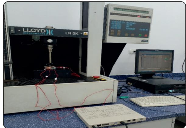
Fig. (7): Strain gauge measurement.
