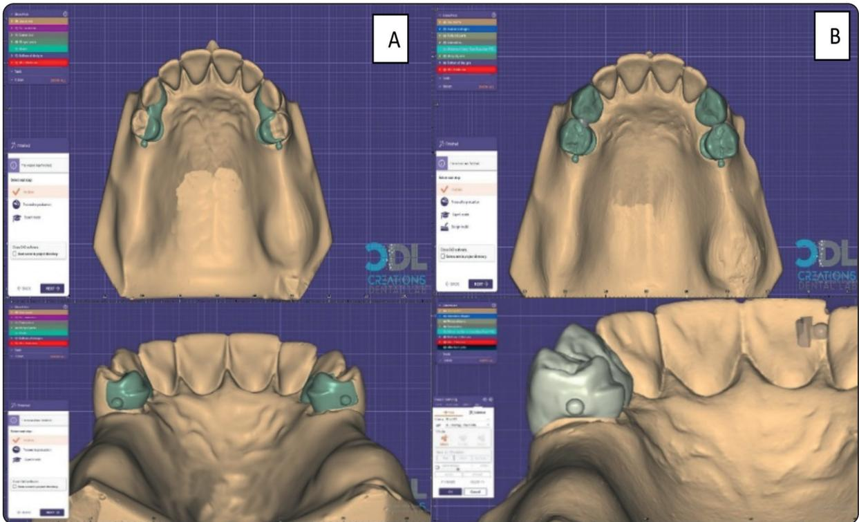
Fig. (3) (A): The virtual model of resin bonded attachment. (B): The virtual model of extracoronary attachment with full veneer retainer (ECFV).
