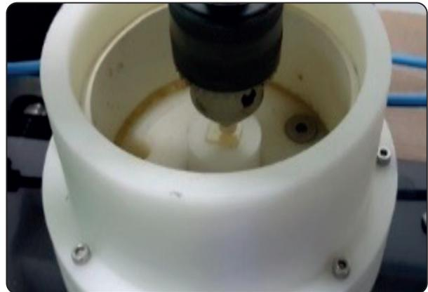
Fig. (2): Ceramic sample embedded in Teflon housing
