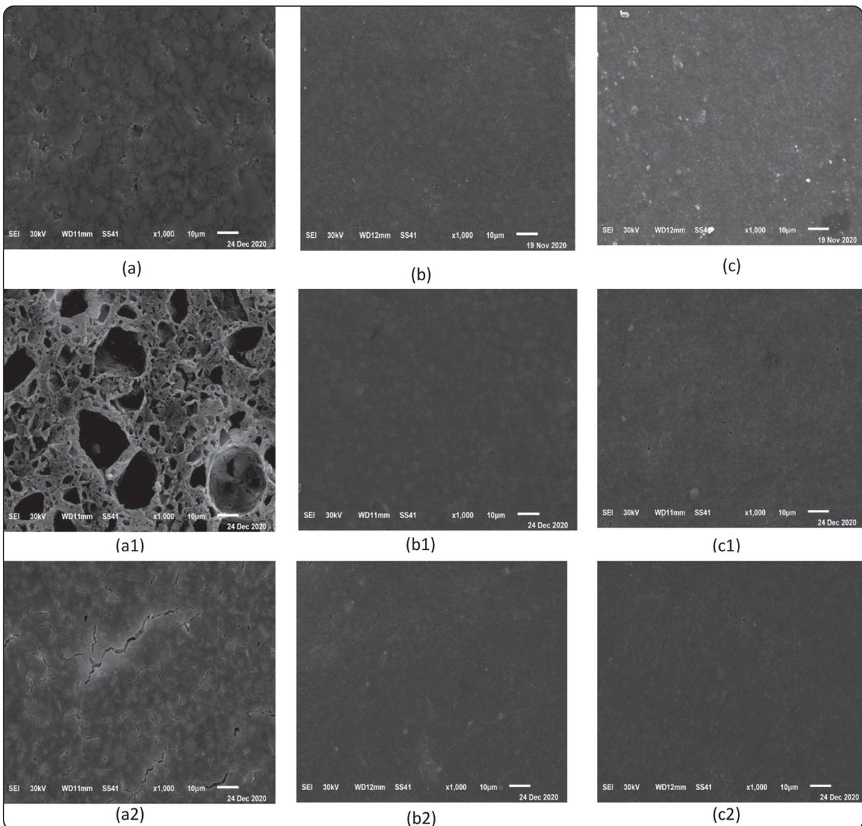
Fig. (2) SEM at magnification 1000x that show surface topography before and after staining. (a) RMGI, (b) micro-hybrid RBC, (c) Nano-hybrid RBC. (a1) RMGI after storage in hibiscus, (b1) micro-hybrid RBC after storage in hibiscus, (c1) micro-hybrid RBC after storage in hibiscus, (a2) RMGI after storage in cinnamon, (b2) micro-hybrid RBC after storage in cinnamon, (c2) Nano-hybrid RBC after storage in cinnamon.
