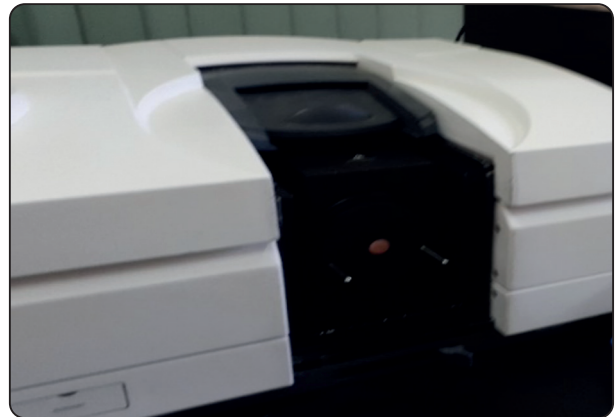
Fig. (2): Sample (Pink Circle) was fixed to the spectrophotometer holder.
