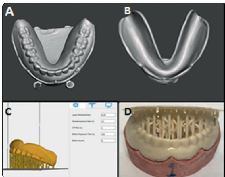
Fig. 3 A,B digitized waxed-up denture, C) planned virtual denture by subtracting, D) 3D-printed denture
