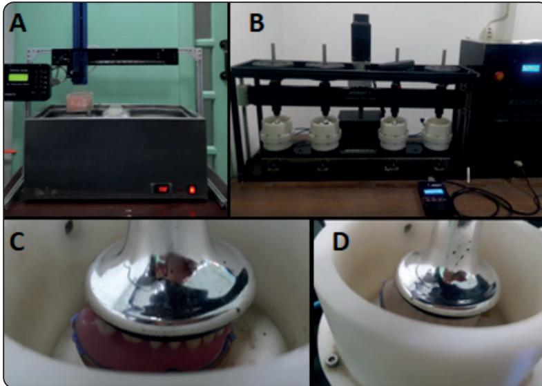
Fig. 4 A, Thermo- cycling procedures, B Four stations multi-modal ROBOTA chewing simulator, C,D mechanical-cycling of conventional and 3D printed dentures
