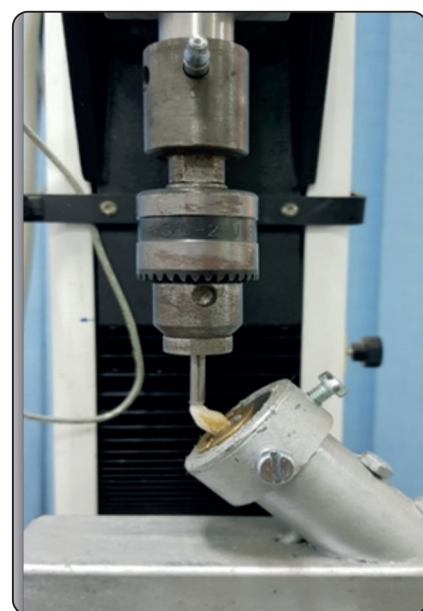
Loading of the tooth at 60^{\circ} angle.
