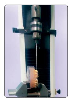
Fig. (3): Typodont mounted on instron testing machine
