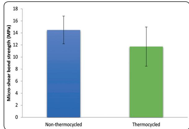
Fig. (2) Bar chart representing mean and standard deviation values for micro-shear bond strength of non-thermocycled and thermocycled specimens regardless of PEEK condition
