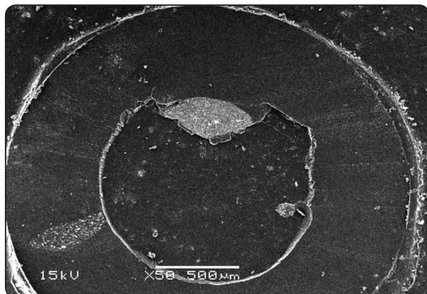
Fig. (6) Topographical analysis of the bonding surface of PEEK totally reprocessed sample showing adhesive mode of failure (50X).
