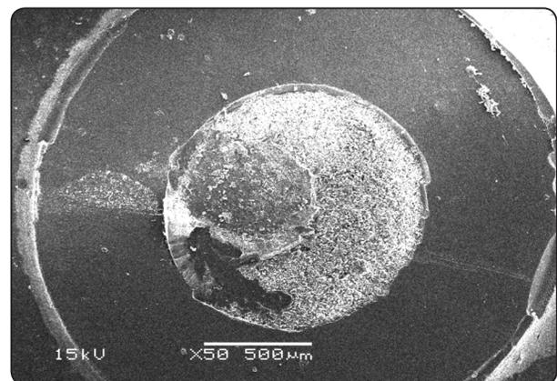
Fig. (5) Topographical analysis of the bonding surface of PEEK partially reprocessed Thermocycled sample showing cohesive mode of failure of cement layer (50X).
