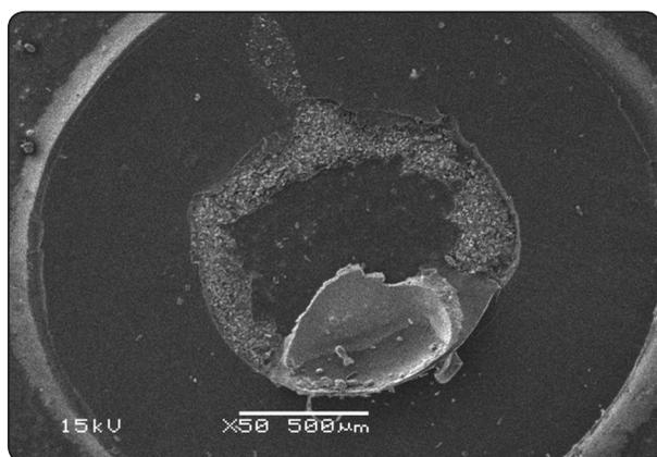
Fig. (7) Topographical analysis of the bonding surface of PEEK totally reprocessed thermocycled sample showing mixed mode of failure (50X).
