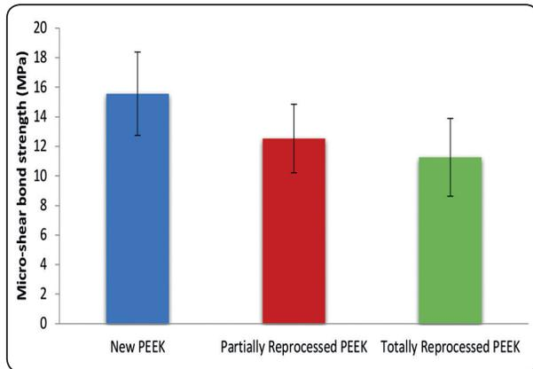
Fig. (1) Bar chart representing mean and standard deviation values for micro-shear bond strength of different PEEK conditions regardless of thermocycling
