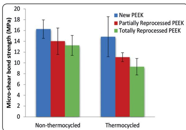
Fig. (3). Bar chart representing mean and standard deviation values for micro-shear bond strength with different interactions of variables
