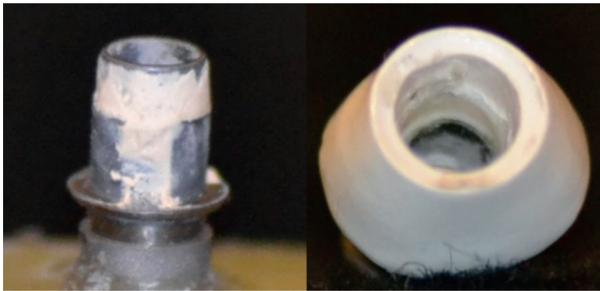
Fig. (11): Failure mode of group V (PEEK Press).
