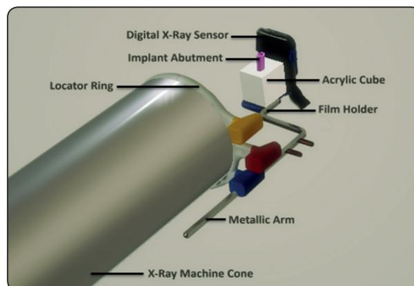
Fig. (1): Diagram showing radiographic imaging set-up.
