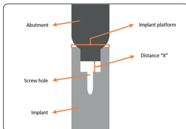
Fig. (2): Schematic diagram showing measurement method. Distance "X" represents the distance from the end of the base of the abutment till the beginning of the screw hole of the implant.
