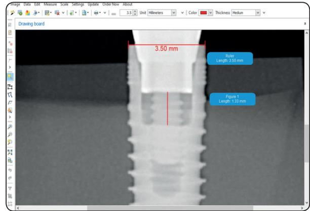
Fig. (6): Radiograph showing representative sample for Group IV: Co-Cr Fully casted Co-Cr abutment.
