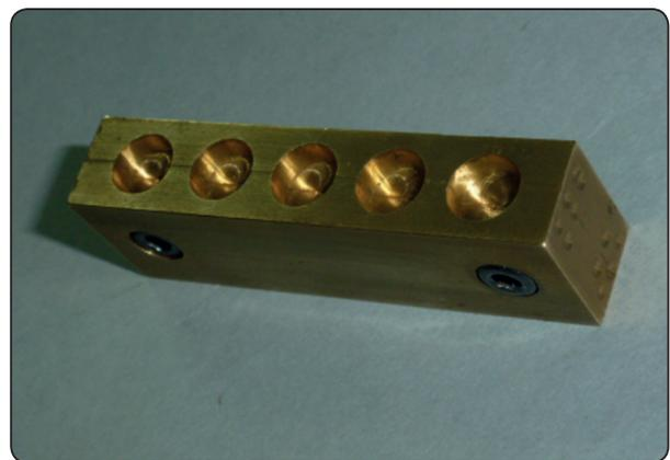
Fig. (1) The copper split mold
