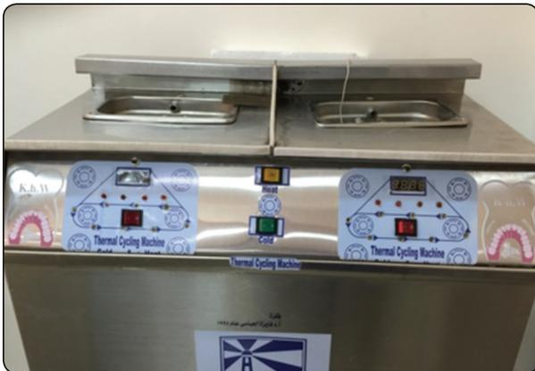
Fig. (3) A custom made Thermocycling machine
