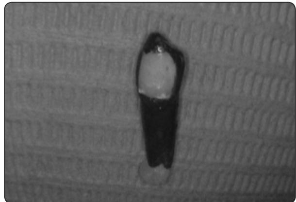
Fig. (4) A specimen coated with nail varnish before immersion in dye.
