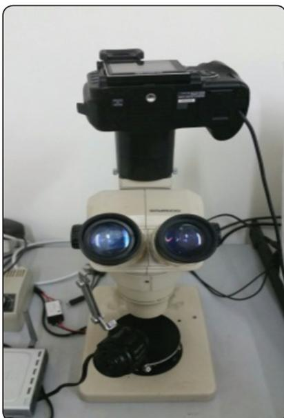
Fig. (5) The stereomicroscope.
