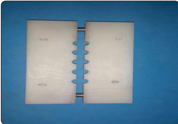
Fig. (1) Showing the mould used to form the sealers cylinders
