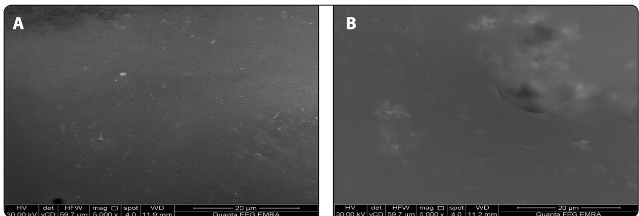
Fig. (6) Representative scanning electron microscope images (X5000) for IPS e.max press Where (A) represents control firing and (B) the 5<sup>th</sup> firing cycle .
