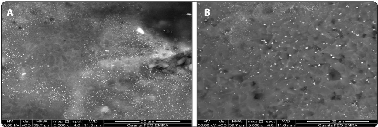
Fig. (7) Representative scanning electron microscope images (X5000) for Celtra press Where (A) represents control firing and (B) the 5<sup>th</sup> firing cycle.
