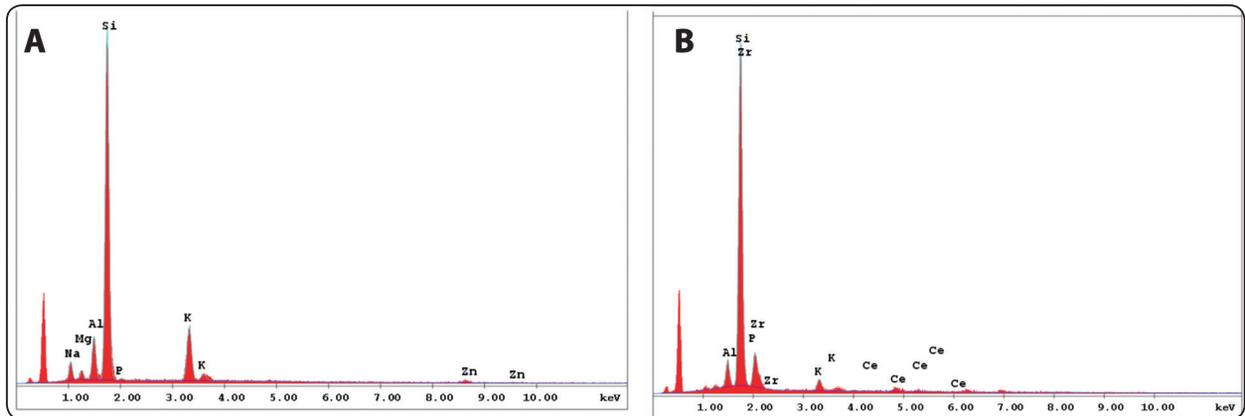
Fig. (10) EDAX for IPS e.max press (A) and Celtra press (B) for control firing group.
