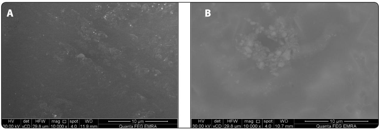
Fig. (8) Representative scanning electron microscope images (X10000) for IPS e.max press Where (A) represents control firing and (B) the 5<sup>th</sup> firing cycle.
