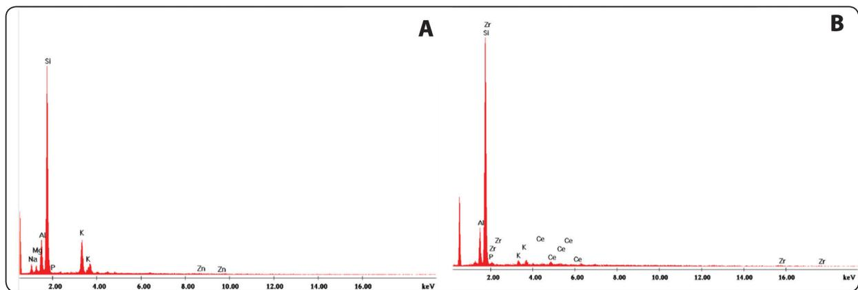
Fig. (11) EDAX for IPS e.max press (A) and Celtra press (B) for 5<sup>th</sup> firing group.
