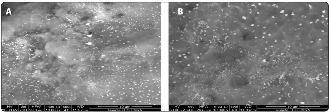
Fig. (9) Representative scanning electron microscope images (X10000) for Celtra press Where (A) represents control firing and (B) the 5<sup>th</sup> firing cycle.
