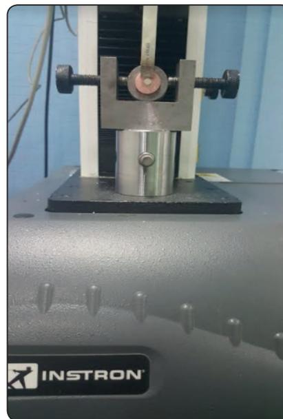
Fig. (1) Showing shear bond strength sample mounted onto testing machine
