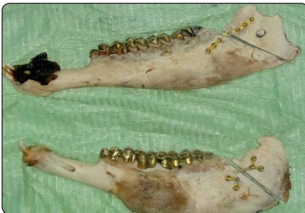
Fig 5: Samples from group A and B showed plating system fractured after loading
