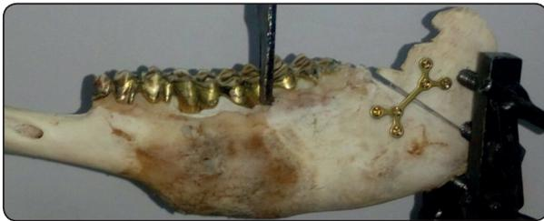
Fig. (3) Prepared model specimen from group A fixed the testing machine
