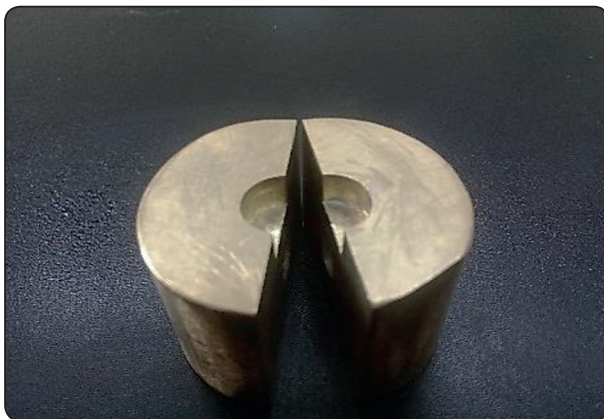
Fig (4). Split copper mold for diametral tensile strength test.
