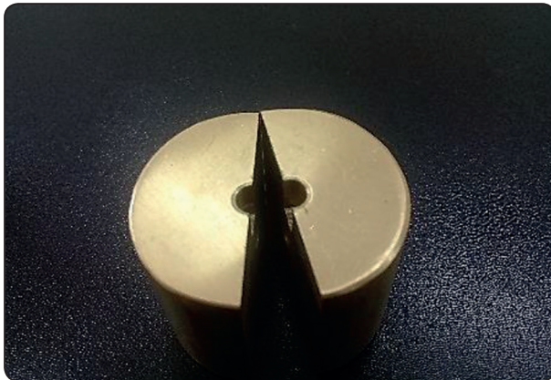
Fig (3). Split copper mold for compressive strength test.
