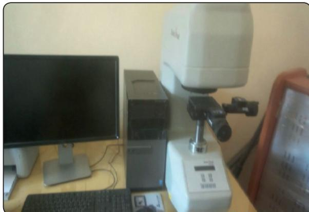
Fig. (1) Indentation hardness tester (Zwick. roell, system 5153. UK).
