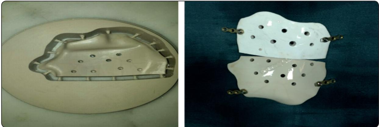
Fig. (3) Photographs showing the printed PEEK prosthetic implant.
